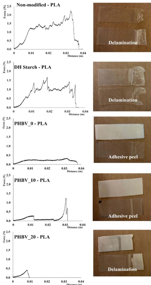
Fig. 3 Typical behaviour of the seal profile and the image of the separation mode of the different bilayers (non-modified starch-PLA, DH starch-PLA, PHBV<sub>0</sub>-PLA, PHBV<sub>10</sub>-PLA and PHBV<sub>20</sub> PLA) during the sealing strength test.
