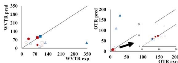
**Fig. 4** Predicted vs. experimental values of WVTR and OTR for different bilayers (blue symbols). Squares represent PLA–starch – full for DH starch and empty for non-modified. Triangles represent PLA–PHBV, with the blue becoming darker as the PEG increased. For trilayers (red symbols), rhombus represents 0% PEG, squares 10% PEG and circles 20% PEG with non-modified starch full symbols and DH empty symbols.
