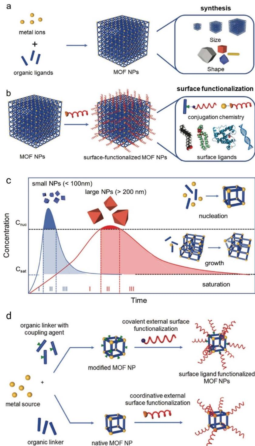
**Fig. 3** Schematic diagram of (a) the controlled synthesis of MOF NPs, (b) the post-synthetic surface modification of the MOF, (c) lamer model of four steps of MOF NP formation, and (d) covalent surface modification (top) and coordinative surface modification (bottom) at the SBUs. Reproduced with permission from Wiley.<sup>44</sup>
