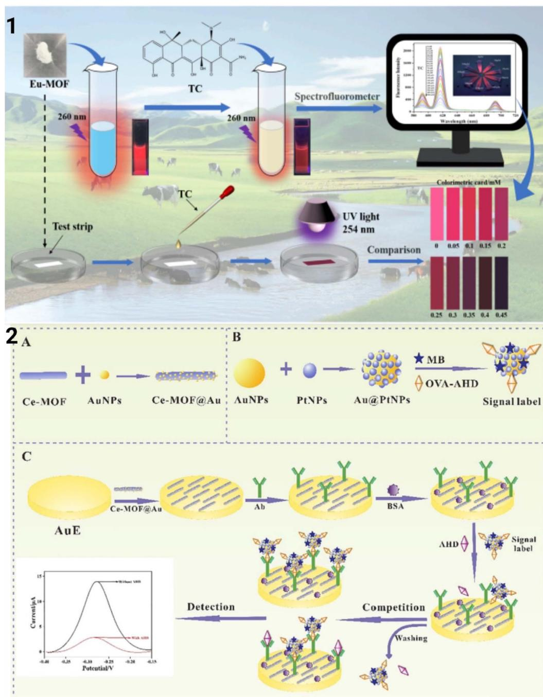
Fig. 10 (1) Eu MOF-based portable test strip for rapid and visual detection of tetracycline based on a simple spectrofluorometer. Reproduced with permission from Elsevier.<sup>87</sup> (2) Detection of nitrofurantoin metabolite 1-aminohydantoin using Ce-MOF@Au by the electrochemical immunosensing technique. Reproduced with permission from Elsevier.<sup>108</sup>
