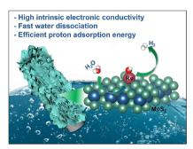
Single-atomic rhenium-assisted 2H-to-1T phase transformation of MoS<sub>2</sub> nanosheets boosting electrocatalytic hydrogen evolution
