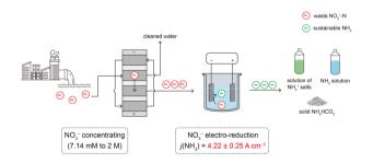
Sustainable waste-nitrogen upcycling enabled by low-concentration nitrate electrodialysis and high-performance ammonia electrosynthesis
