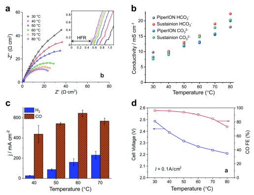
Fig. 7 Effect of heating on CO<sub>2</sub> electrolyzers. Effects of temperature on (a) the impedance, (b) ionic conductivity, (c) current density and (d) product selectivity of the electrolyzer. Proper temperature facilitates ion transport, reduces impedance, and increases current density. (a) and (d) Reproduced with permission from ref. 43, 47 copyright 2019, RSC Publishing. (b) and (c) Reproduced with permission from ref. 47 copyright 2020, RSC Publishing.
