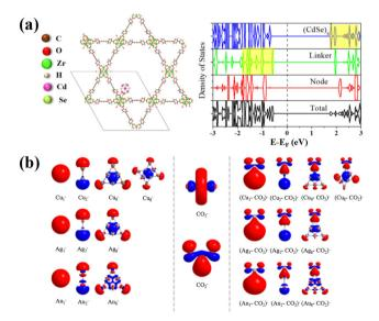
Fig. 2 (a) Structure of the Cd<sub>6</sub>Se<sub>6</sub> cluster encapsulated in NU-1000 at a node site (Cd<sub>6</sub>Se<sub>6</sub>@NU-1000); total and partial density of states of  $Cd_6Se_6@NU-1000$ . (b) HOMOs of  $M_n^-$  clusters, LUMO of  $CO_2$  (top) and HOMO of  $CO_2^-$  (bottom), and HOMOs of  $(M_n-CO_2)^-$  complexes calculated by B3LYP functional (M = Cu, Ag, Au; n = 1, 2, 6 (and 8 for Cu)). Reproduced from ref. 66 and 67 with permission from the American Chemical Society
