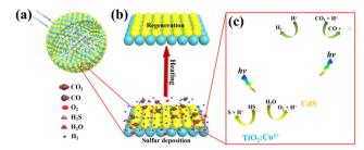
Fig. 3 (a) The complex scattering of light in the CdS/TiO $_2$ :Cu (CTC) hollow spheres. (b) Regeneration of the catalyst by heat treatment desulfurization. (c) The step-scheme charge transfer diagram between CdS and TiO<sub>2</sub>:Cu, as well as the redox reactions of the gaseous adsorbates under the full spectrum of xenon lamp. Reproduced from ref. 24 with permission from Wilev-VCH.
