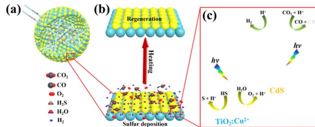
Fig. 3 (a) The complex scattering of light in the CdS/TiO<sub>2</sub>:Cu (CTC) hollow spheres. (b) Regeneration of the catalyst by heat treatment desulfurization. (c) The step-scheme charge transfer diagram between CdS and TiO<sub>2</sub>:Cu, as well as the redox reactions of the gaseous adsorbates under the full spectrum of xenon lamp. Reproduced from ref. 24 with permission from Wiley-VCH.
