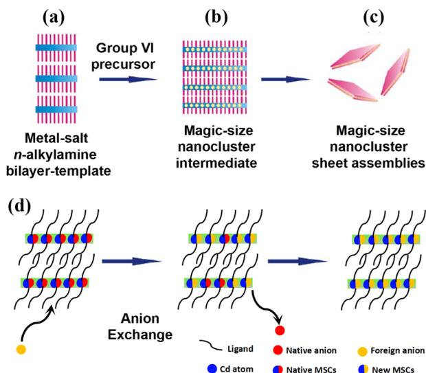
**Fig. 1** (a) The combination of metal salts and primary-amine solvents forms lamellar, primary-amine-bilayer templates. (b) The addition of group VI precursors results in the growth of magic-size nanoclusters within the templates. (c) Ligand exchange with oleylamine liberates sheetlike aggregates. (d) Formation of new MSCs via an anion exchange pathway. Reproduced from ref. 48 and 49 with permission from the American Chemical Society.
