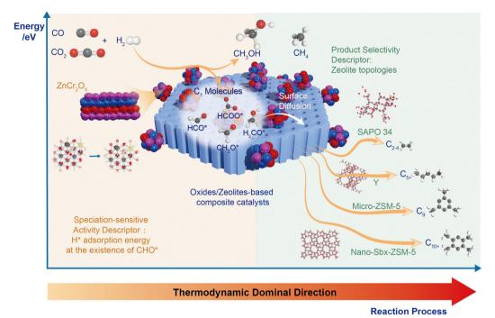
Schematical diagram of bifunctional catalysts and corresponding activity and selectivity descriptor.
