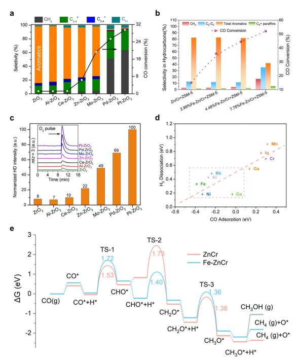
Fig. 2 The modulation on metal oxides in syngas to aromatics. (a) Effect of metal doping on the catalytic performance of M-ZrO<sub>2</sub>/H-ZSM-5 (M denotes metal oxides). Reprinted with permission. Copyright 2019 Chemistry Europe. (b) Catalyst evaluation of pristine  $ZnCr_2O_4$  and different  $ZnCr_2O_4$  and d
