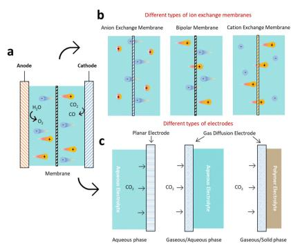
Fig. 2 Schematic diagram of ECR device and influencing factors. (a) A typical ECR system. The anodic and cathodic electrocatalysts perform oxidation and reduction reactions, respectively. (b) The membrane separates the cathodic and anodic compartments. (c) Three different types of electrodes for ECR.
