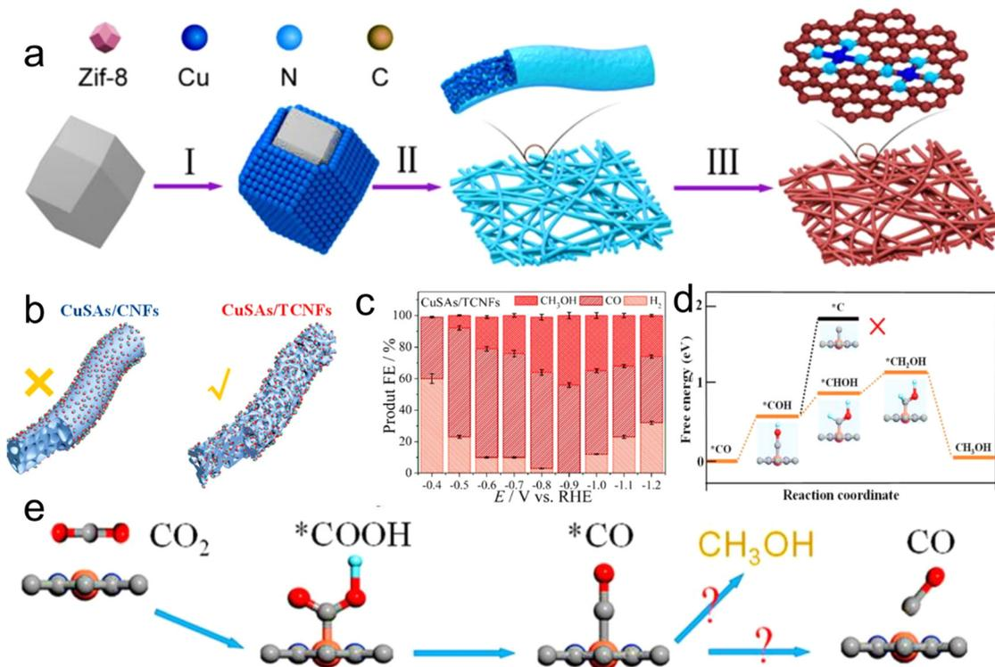
Fig. 22 (a) Synthesis of Cu single atom. (b) Illustration of CO<sub>2</sub> diffusion on two samples. (c) FEs of products. (d) Free energy model for the conversion of \*CO to methanol. (e) Optimized atomic structures of CuSAs/TCNFs and proposed reaction paths for CO<sub>2</sub> electroreduction. Reproduced with permission from ref. 206 Copyright 2019, ACS.
