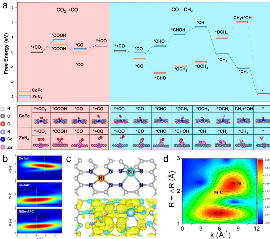
Fig. 29 (a) Free energy profiles and intermediate configuration over CoPc and ZnN<sub>4</sub>. Reproduced with permission from ref. 20 Copyright 2020, Wiley. (b) WT analysis of NiSn-APC, Sn-SAC and Sn foil. (c) Spin electron density model proposed for NiSn-APC (yellow; spin up and green; spin down). Reproduced with permission from ref. 261 Copyright 2021, Wiley. (d) WT-EXAFS plot for Ni-CNC-1000. Reproduced with permission from ref. 262 Copyright 2022, Wiley.
