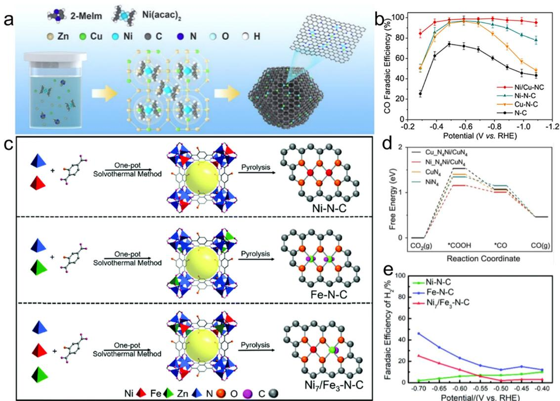
Fig. 24 (a) Schematic description of Ni/Cu–N–C fabrication. (b)  $FE_{CO}$ . Reproduced with permission from ref. 233 Copyright 2022, ACS. (c) Method for the synthesis of different metal-based catalysts. Reproduced with permission from ref. 234 Copyright 2021, RSC. (d) Free energy diagram for CO<sub>2</sub> conversion. Reproduced with permission from ref. 233 Copyright 2022, ACS. (e) FE of H<sub>2</sub> for various catalysts. Reproduced with permission from ref. 234 Copyright 2021 RSC.
