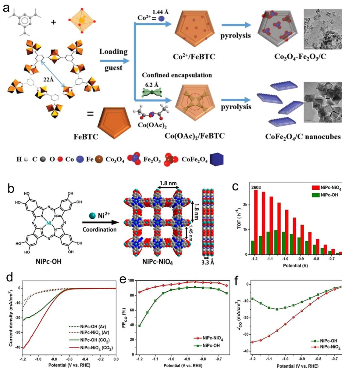
Fig. 2 (a) Illustration of assembly MOF-derived bimetallic spinel oxide  $\text{CoFe}_2\text{O}_4$  nanocubes through the combination of exchange-coordination and pyrolysis. Reproduced with permission from ref. 58 Copyright 2020, Wiley. (b) Synthesis. (c) Turnover frequency. (d) LSV curves in  $\text{CO}_2$ . (e) FEs for  $\text{CO}$ . (f)  $\text{CO}$  partial current density of  $\text{NiPc-NiO}_4$ . Reproduced with permission from ref. 59 Copyright 2021, Wiley-VCH.
