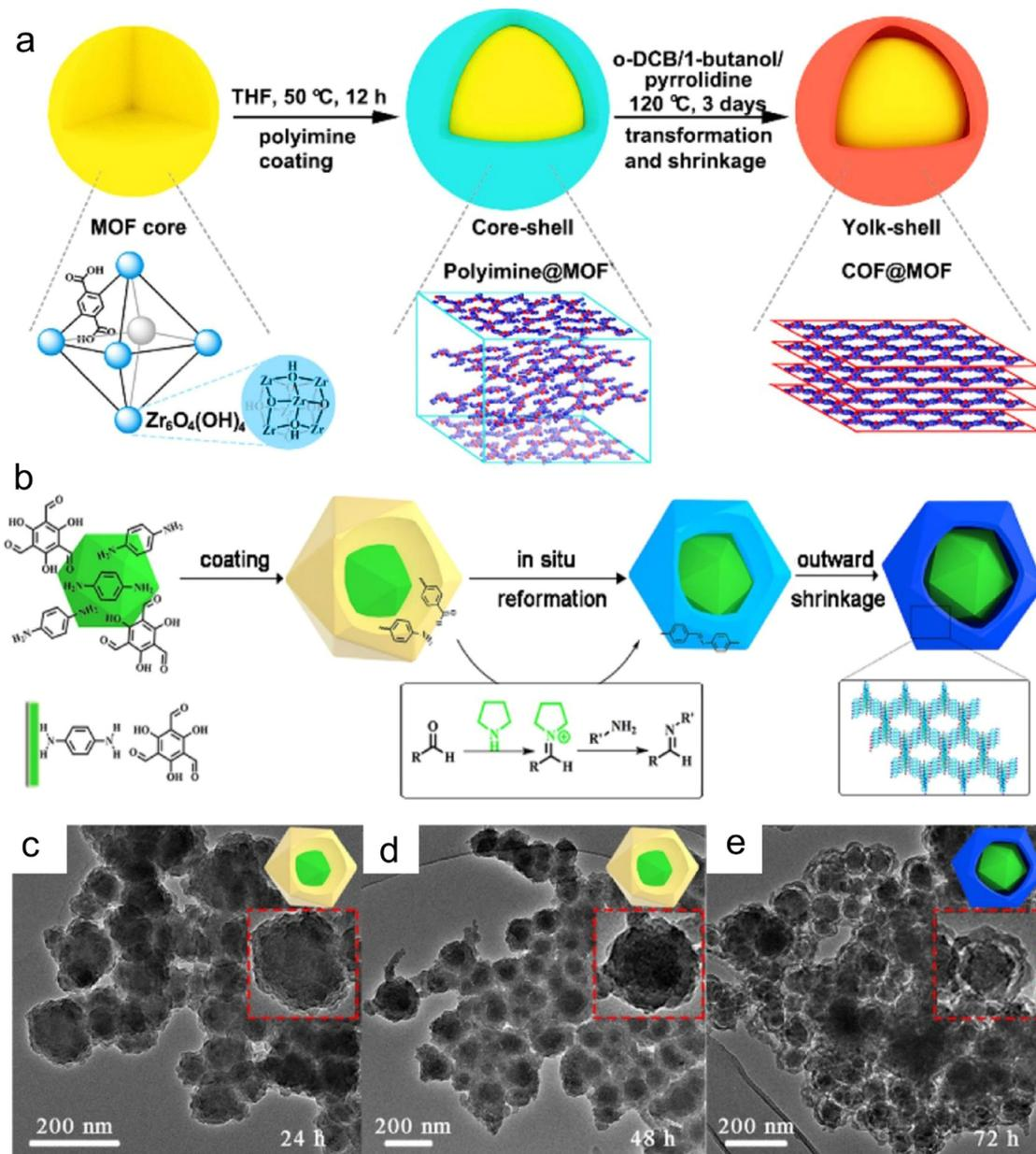
Fig. 3 (a) Synthesis of yolk shell COF@MOF nanocomposites and the *in situ* transformation of the COF shell. (b) Proposed mechanism of the formation of yolk-shell-structured COF@MOF. (c–e) Time-dependent experiments of YS-TpPa@UiO-66-(COOH)<sub>2</sub>. Reproduced with permission from ref. 60 Copyright 2021, ACS.
