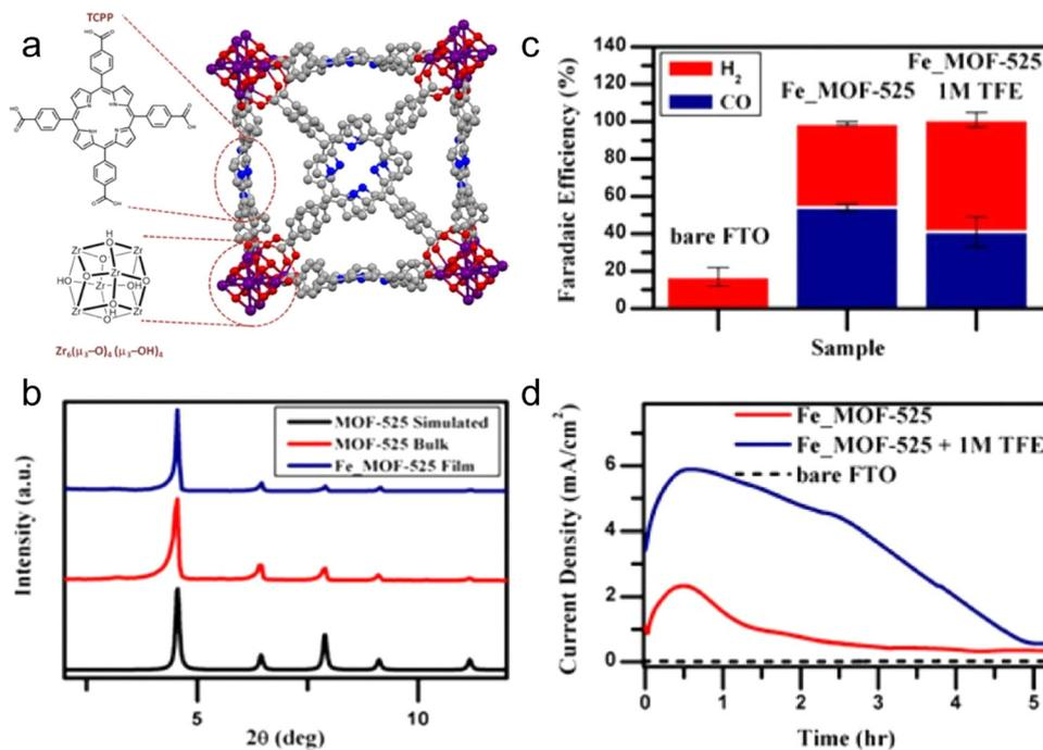
Fig. 8 (a) Crystal structure of MOF-525 including the chemical structure of Zr-based node. (b) Comparison of PXRD of Fe-MOF-525 and other MOFs. (c) FE. (d) Current density vs. time. Reproduced with permission from ref. 123 Copyright 2015, ACS.
