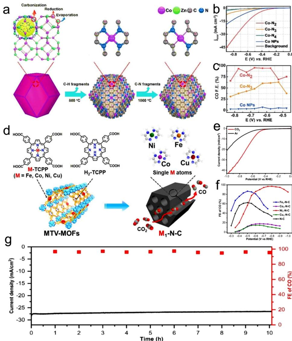
Fig. 16 (a) Co-N<sub>4</sub> synthesis process. (b) LSV curves of all the materials and (c) FEs. Reproduced with permission from ref. 181 Copyright 2021, Wiley. (d) Synthesis of M<sub>1</sub>-N-C single-atom catalysts. (e) LSV curves of Ni<sub>1</sub>-N-C. (f) FEs and (g) durability test of Ni<sub>1</sub>-N-C. Reproduced with permission from ref. 182 Copyright 2020, Wiley-VCH.
