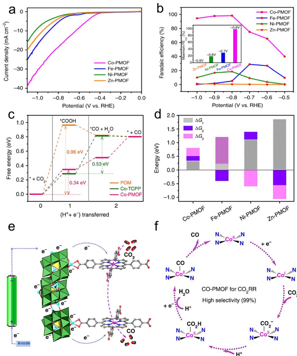
Fig. 14 (a) LSV curves of PMOFs. (b) FEs. (c) Free energy diagram. (d) Free energy comparison of elementary reactions. (e and f) Suggested mechanism for the CO<sub>2</sub>RR on Co-PMOF. Reproduced with permission from ref. 168 Copyright 2018, Springer Nature.
