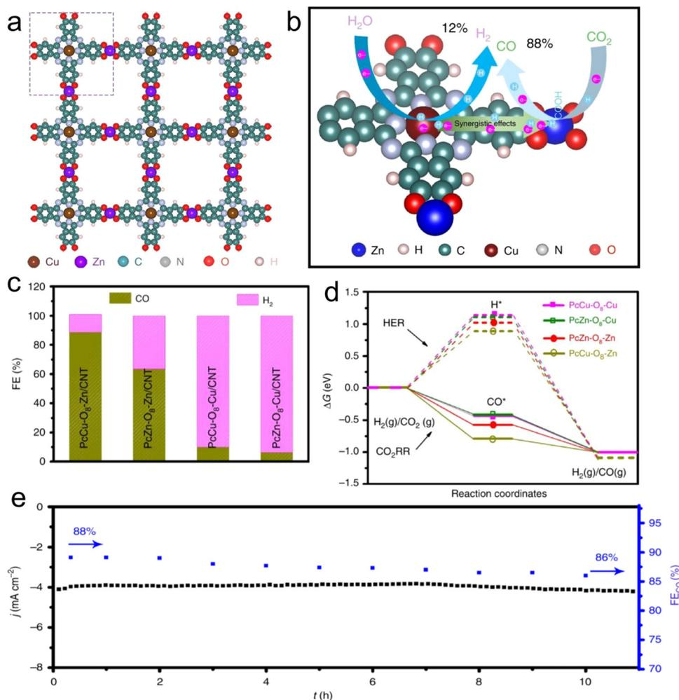
**Fig. 19** (a) Illustration of the crystal structure of Zn-PcCu-O<sub>8</sub>. (b) Depiction of CO<sub>2</sub>RR and HER over Zn-PcCu-O<sub>8</sub>. (c) FEs of H<sub>2</sub> and CO for different catalysts. (d) Possible free energy diagram for different catalysts. (e) Amperometry (*i* ~ *t*) stability test for Zn-PcCu-O<sub>8</sub>/CNT. Reproduced with permission from ref. 189 Copyright 2020, Springer Nature.
