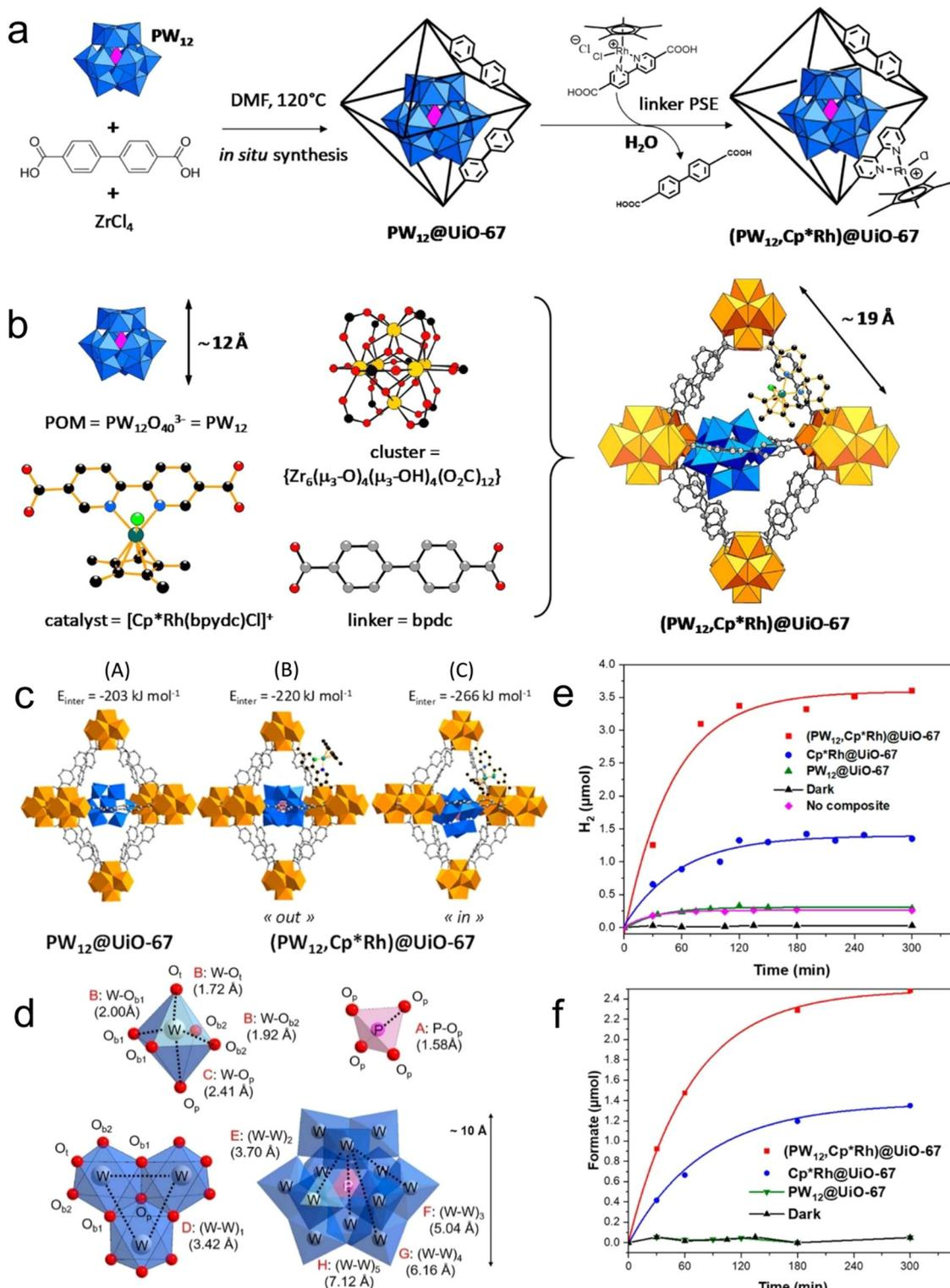
Fig. 11 (a) Schematic of *in situ* synthesis. (b) Components of  $(PW_{12}, Cp^*Rh)@UiO-67$ . (c) Models of  $PW_{12}@UiO-67$  and  $(PW_{12}, Cp^*Rh)@UiO-67$ . (d) Distances between the components of POM. Production rate of (e)  $H_2$  and (f)  $HCOO^-$ . Reproduced with permission from ref. 166 Copyright 2020, ACS.
