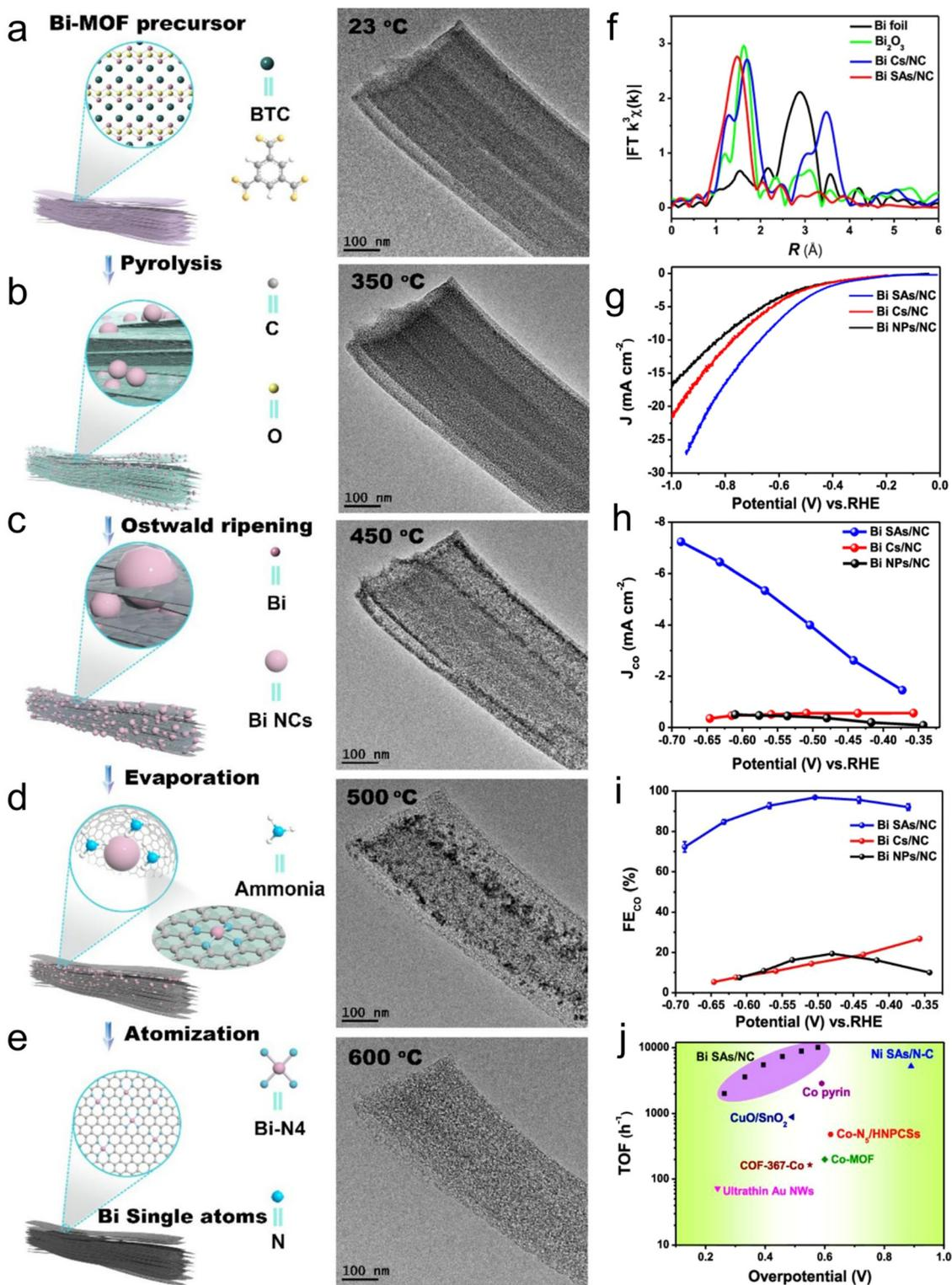
Fig. 23 (a–e) Illustration of the transformation of Bi-MOF to Bi-SA together with corresponding TEM images. (f) EXAFS spectra with  $k^3\chi(k)$  function. (g) LSV curves. (h) Partial current densities of CO. (i) FE<sub>CO</sub> and (j) comparison of TOF values. Reproduced with permission from ref. 212 Copyright 2019, ACS.
