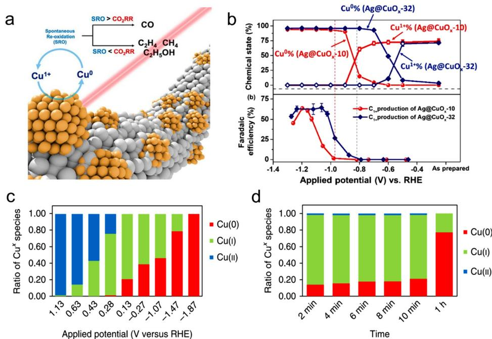
Fig. 7 (a) Schematic process of Cu during the CO<sub>2</sub>RR. (b) FE and chemical state vs. applied potential. Reproduced with permission from ref. 120 Copyright 2019, ACS. (c) Oxidation state ratio of Cu vs. applied potential. (d) Oxidation state ratio vs. time. Reproduced with permission from ref. 121 Copyright 2018, Springer Nature.
