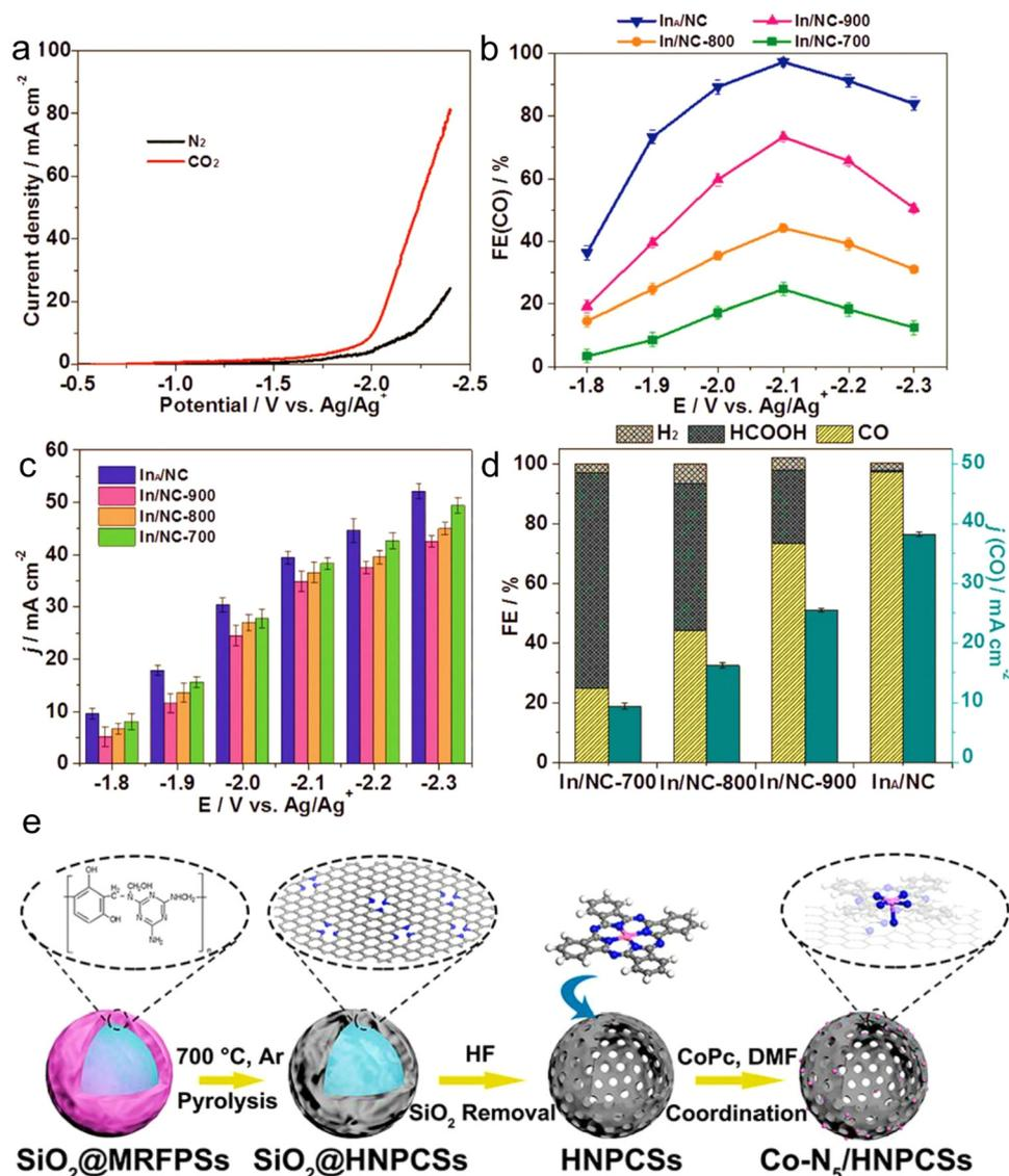
Fig. 26 (a) LSV curves for In<sub>n</sub>/NC catalyst. (b) FEs and (c) partial current densities over for CO. (d) FEs of formate, H<sub>2</sub> and CO. Reproduced with permission from ref. 238 Copyright, 2021 ACS. (e) Schematic of the synthesis of Co-N<sub>5</sub>/HNPCs. Reproduced with permission from ref. 241 Copyright 2018, ACS.
