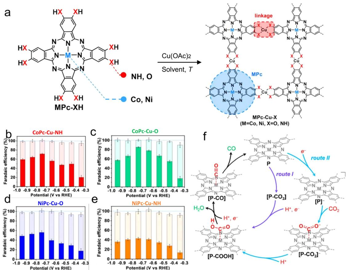
Fig. 25 (a) Synthesis scheme of MPC-Cu-X MOFs. (b–e) FEs of H<sub>2</sub> product for different (catalysts). (f) Suggested mechanism for catalytic electrochemical reduction of CO<sub>2</sub> to CO on MPC-Cu-XH MOFs. Reproduced with permission from ref. 236 Copyright 2020, ACS.
