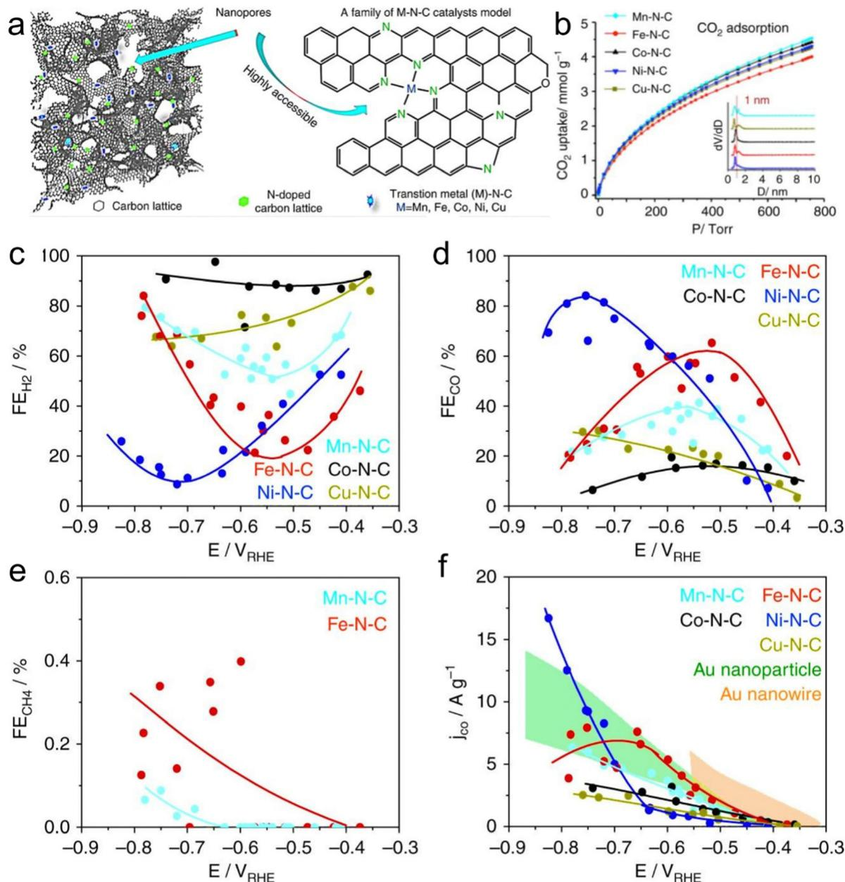
Fig. 17 (a) M–N–C model and structure. (b) Adsorption isotherm curves for CO<sub>2</sub> and inset is the pore size distribution. (c–e) FEs of H<sub>2</sub>, CO and CH<sub>4</sub>, respectively. (f) Mass-normalized partial currents for CO. reproduced with permission from ref. 183 Copyright 2017, Springer Nature.
