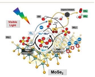
Fig. 8 Proposed mechanisms for the visible-light-driven MoSe<sub>2</sub>/PMS system. Copied with permission from ref. 5. Copyright 2021, Elsevier.
