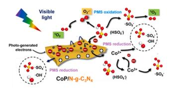
Fig. 6 The proposed mechanism in the CoP/N-g-C<sub>3</sub>N<sub>4</sub> nanosheets catalyzed visible-light-driven PMS activation. Copied with permission from ref. 33. Copyright 2021, Elsevier.
