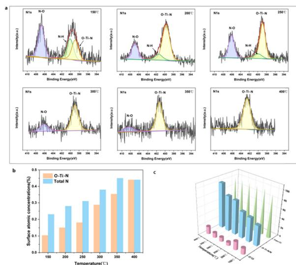
Fig. 2 The *in situ* XPS spectra obtained from the  $\text{H-TiO}_{2-x}$  during the  $\text{NH}_3$ -SCR process at 150–400 °C. (a) N1s. (b) Surface N atom concentrations and O–Ti–N concentrations at various temperatures. (c) Percentage content of the active components O, N and Ti ( $\text{O}' = \text{O}_\beta + \text{O}_\gamma$ ).
