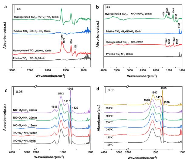
Fig. 5 The DRIFT spectra obtained from the hydrogenated  $\text{TiO}_{2-x}$  and pristine  $\text{TiO}_2$ . (a) NO and  $\text{O}_2$  followed by  $\text{NH}_3$  at  $300 \text{ }^\circ\text{C}$ . (b)  $\text{NH}_3$  followed by NO +  $\text{O}_2$  at  $300 \text{ }^\circ\text{C}$ . (c)  $\text{NH}_3$  + NO +  $\text{O}_2$  for 30 min at  $300 \text{ }^\circ\text{C}$ . (d)  $\text{NH}_3$  + NO +  $\text{O}_2$  with a temperature gradient.
