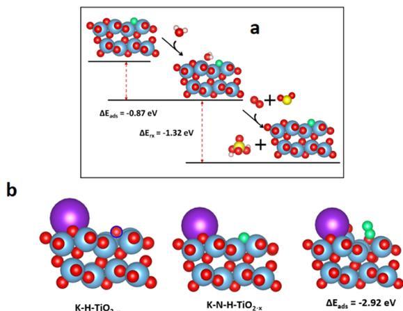
Fig. 7 (a) Reaction coordinates of adsorption of water followed by SO<sub>2</sub> on N-H-TiO<sub>2-x</sub>, and (b) adsorption of K on H-TiO<sub>2-x</sub> and N-H-TiO<sub>2-x</sub> and NO adsorption on K-N-H-TiO<sub>2-x</sub>. Legend: red = O; blue = Ti; pink = H; green = N; yellow = S; purple = K; and blue circle = oxygen vacancy.
