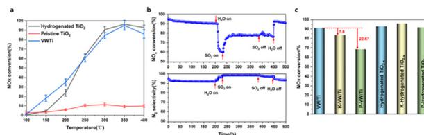
Fig. 1 NH<sub>3</sub>-SCR denitrification activity of the catalyst. (a) The denitrification performances of pristine TiO<sub>2</sub>, H-TiO<sub>2-x</sub> and VW/Ti catalysts. (b) Data from 500 h durability trials with the H-TiO<sub>2-x</sub> catalyst at 350 °C. (c) Tolerance of K<sub>2</sub>O and P<sub>2</sub>O<sub>5</sub> of the H-TiO<sub>2-x</sub> catalyst and of commercial VW/Ti catalysts at 350 °C.
