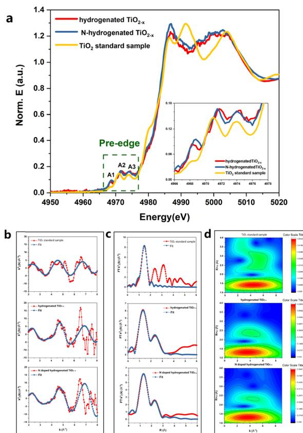
Fig. 3 The XANES spectra of the catalyst samples before and after the SCR reaction. (a) The Ti K-edge, (b) extended region fitting using ARTEMIS in R-space, (c) fitted magnitude of  $k_2$ -weighted Ti K-edge EXAFS spectra, and (d) wavelet transform images obtained for the  $\text{TiO}_2$  standard sample (anatase), hydrogenated  $\text{TiO}_{2-x}$  and N-hydrogenated  $\text{TiO}_{2-x}$ .
