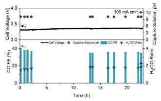
Fig. 4 Long-term operation of DCE over 23 hours with CO FE, H<sub>2</sub>/CO ratio, full cell voltage, and capture solution pH noted. Experiment conducted at a constant current density of 100 mA cm<sup>-2</sup> with a 1 cm<sup>2</sup> active area. Schematic and picture of the experimental set-up are provided in the ESI† (Fig. S10A and B).
