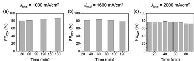
Fig. 5  $FE_{C_{2+}}$  stability tests with respect to the current density over CuONPs-1.0/GDE in 1 M KCl under (a)  $J_{total} = 1000 \text{ mA cm}^{-2}$ , (b)  $1600 \text{ mA cm}^{-2}$  and (c)  $2000 \text{ mA cm}^{-2}$ .
