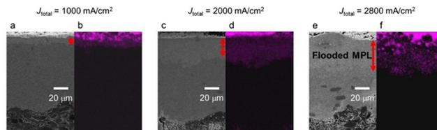
Fig. 3 (a, c and e) Cross-sectional SEM images of CuONPs-1.7/GDE and (b, d and f) K<sup>+</sup> distribution (purple) obtained by EDX after application of  $J_{total} = (a \text{ and } b) 1000 \text{ mA cm}^{-2}$ , (c and d)  $2000 \text{ mA cm}^{-2}$ , and (e and f)  $2800 \text{ mA cm}^{-2}$  for 30 min under CO<sub>2</sub>RR conditions in 1 M KCl.
