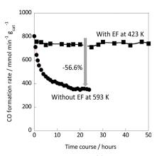
Fig. 3 Catalytic stability during the RWGS reaction over the Ru(col)/ $ZrTiO_4$  catalyst with/without the electric field (5 mA);  $CO_2: H_2: Ar = 1:1:2$ ; total flow rate: 100 SCCM; 100 mg catalyst weight.
