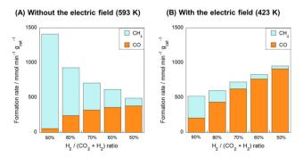
Fig. 4 CO and CH $_4$  formation rate over the Ru(col)/ZrTiO $_4$  catalyst under various H $_2$ /CO $_2$  ratios (A) without the electric field at 593 K and (B) with the electric field (5 mA) at 423 K; 100 SCCM total flow rate; 100 mg catalyst weight.
