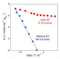
Fig. 2 Arrhenius plots for the RWGS reaction over the Ru(col)/ZrTiO $_{4}$ catalyst with and without the electric field;  $CO_2:H_2:Ar = 1:1:2;$ 100 SCCM total flow rate; 100 mg catalyst weight; 0 or 5.0 mA imposed
