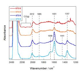
Fig. 5 In situ DRIFTS spectra under the RWGS reaction atmosphere over the Ru(col)/ZrTiO<sub>4</sub> catalyst without the electric field at 373-673 K; CO<sub>2</sub>:  $H_2: Ar = 1:1:2;$  40 SCCM total flow rate
