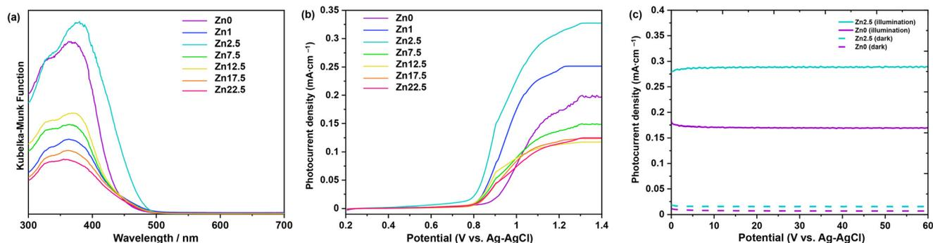
Fig. 5 (a) UV-vis diffuse reflectance spectra of  $\text{Bi}_{2-x}\text{Zn}_x\text{WO}_{6+\delta}$  powders with varying contents of  $\text{Zn}^{2+}$  substituent. Photoelectrochemical results of  $\text{Bi}_{2-x}\text{Zn}_x\text{WO}_{6+\delta}$  as photoanodes in 0.1 M  $\text{Na}_2\text{SO}_4$  deoxygenated water solution: LSV (b) and CA (c) at 1.4 V (V vs. Ag-AgCl) for Zn0 and Zn2.5.
