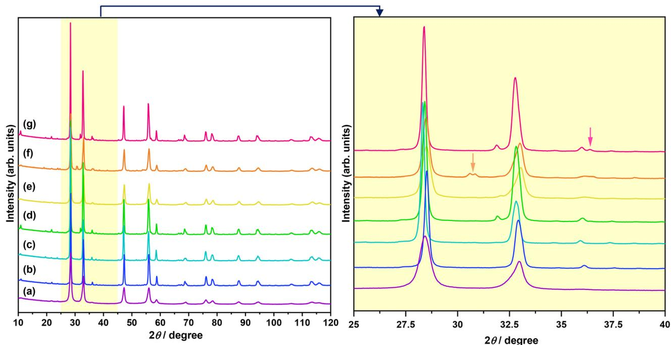
Fig. 1 XRD patterns of  $\text{Bi}_{2-x}\text{Zn}_x\text{WO}_{6+\delta}$  powders with varying contents of  $\text{Zn}^{2+}$  substituent: (a) Zn0, (b) Zn1, (c) Zn2.5, (d) Zn7.5, (e) Zn12.5, (f) Zn17.5, and (g) Zn22.5. The orange and magenta arrows indicate the reflections belonging to  $\text{ZnWO}_4$  and  $\text{ZnO}$ , respectively.
