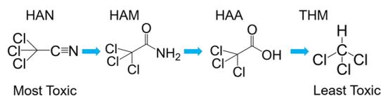
Fig. 1 Example reaction scheme showing hydrolysis of trichloroacetone nitrile to chloroform. Note that the initial reaction is substantially faster than the following two.
