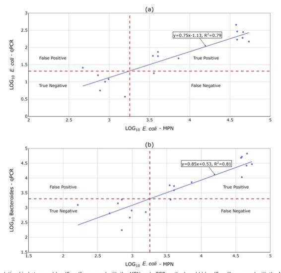
Fig. 6 The relationship between a) log (E. coli) measured with the MPN and gPCR method, and b) log (E. coli) measured with the MPN method and log (Bacteroides) measured with the qPCR method. The red dashed lines indicate the limit values of hygienic safety.
