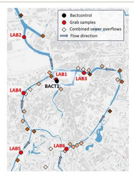
Fig. 1 The canal system of Breda including the locations of measurements and of combined sewer overflows (darker color indicates a higher discharge potential). Culture-based measurements were performed at numbered sites LAB 1-LAB 6. The BACTcontrol was used at location BACT 1, approximately the same as LAB 1.
