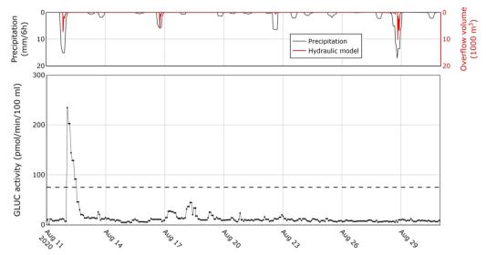
Fig. 4 GLUC activity recorded by the BACTcontrol between 11 and 31 August 2020. The above graph includes the 6-hour sum of precipitation *via* radar measurements and the overflow volume simulated with InfoWorks®. The black dashed line shows the established hygienic limit values for GLUC activity.
