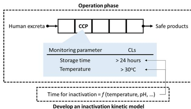
**Fig. 1** Implementation of the HACCP approach to a process train for resource recovery from human excreta. A process train is composed of sequential treatment units, including sedimentation, dewatering, stabilization of readily degradable organic matter, and storage. A critical control point (CCP) identified among the continuous processes is monitored with monitoring parameters so that they meet the critical limits (CLs).
