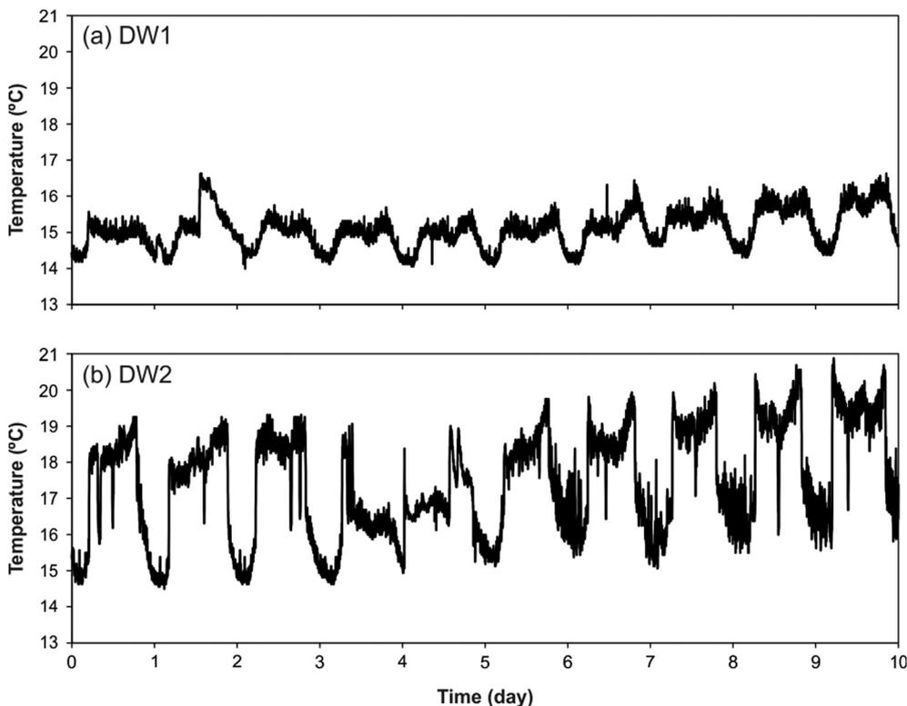
Fig. 2 Wastewater temperature measurements under DWF conditions downloaded from the UWO repository:<sup>26</sup> DW1 (a) and DW2 (b).
