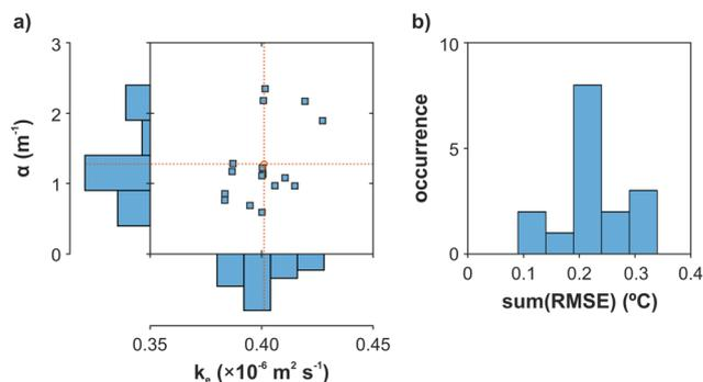
**Fig. 6** Calibrated sediment thermal diffusivity and leakage coefficient (mean  $k_e$  and  $\alpha$  values are marked with a red circle and dashed lines) (a), and overall performance of the 16 steps cross validation process (b).
