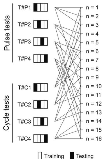
**Fig. 3** Cross-validation procedure. For example, step  $n = 16$  took T#P4 and T#C4 from the pulse and cycle experiment configurations, respectively. In both configurations, results from 2, 4, and 6 cm sediment thickness experiments were applied to calibrate the model, and results from 8 cm sediment thickness experiments were applied to test its performance.
