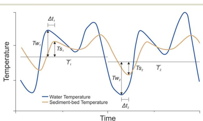
**Fig. 5** Local max/min method scheme (based on Luce *et al.*, 2013).<sup>19</sup> Definition for time differences ( $\Delta t_1$  and  $\Delta t_2$ ) and temperature ratios ( $T_{s1}/T_{w1}$  and  $T_{s2}/T_{w2}$ ) between local maxima and minima. Note that the sketch for the daily mean temperatures was simplified as these values might not coincide for liquid and sediment-bed time series.
