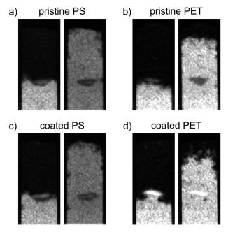
**Fig. 3** Neutron images during and at the end of capillary rise of water. The hotspots consist of (a) pristine PS, (b) pristine PET, (c) Fh-coated PS, and (d) Fh-coated PET. For each set, the left image is taken at a time step at which the rising water reaches the hotspot. For coated PET, water flow into the hotspot is observed whereas for the other variants, the water bypasses the hotspot. The right image of each set is taken at the end of capillary rise (150 s).
