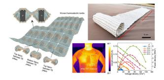
Scalable manufacturing of a durable, tailorable, and recyclable multifunctional woven thermoelectric textile system
