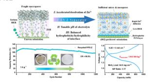
Highly-reversible and recyclable zinc metal batteries achieved by inorganic/organic hybrid separators with finely tunable hydrophilichydrophobic balance
