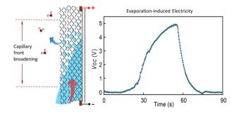
Capillary front broadening for water-evaporationinduced electricity of one kilovolt
