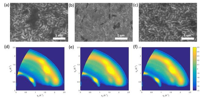
Fig. 3 SEM micrographs of the reference perovskite film (a) and of the samples treated with SnAc<sub>4</sub> + DMS (b) and SnAc<sub>2</sub> + DMS (c). (d)-(f) GIWAXS patterns of the corresponding three different perovskite films recorded using an incident angle of 0.5°.
