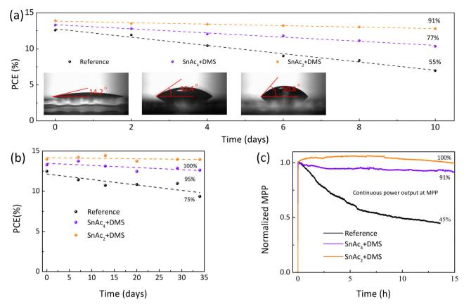
Fig. 6 (a) Air stability (30-40% humidity) of non-encapsulated quasi-2D Pb-Sn solar cells, the inset shows the contact angle of three corresponding active layer with passivation. Storage stability (b) and operational stability (c) of non-encapsulated devices in a  $N_2$ -filled glovebox. The operational stability is measured at the MPP under continuous 1 sun, AM1.5G illumination.
