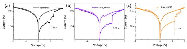
Fig. 5 Typical J-V curves of reference (a),  $SnAc_4 + DMS$  (b), and  $SnAc_2 + DMS$  (c)-treated memory devices.
