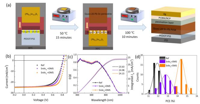
Fig. 1 (a) Schematic diagram of the preparation of quasi-2D Pb-Sn perovskite with a two-steps blade coating process. (b) J-V curves of the bestperforming PSCs. (c) EQE spectra and integrated photocurrent of the devices. (d) Statistical distribution of PCEs for the three different sample types.
