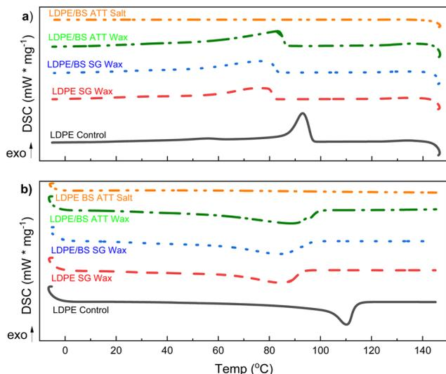
Fig. 9 Differential scanning calorimetry (DSC) data on the solid waxy condensable products from both SG and ATT reactions to compare the efficacy of the crystallization and melting behaviors of the polymeric products with respect to the original LDPE. DSC heating curves (a) and cooling curves (b) were collected in argon atmospheres for SG of LDPE, SG of LDPE/BS, and ATT of LDPE/BS. The salt from the latter ATT reaction (LDPE/BS ATT) was tested for residual polymeric matter.
