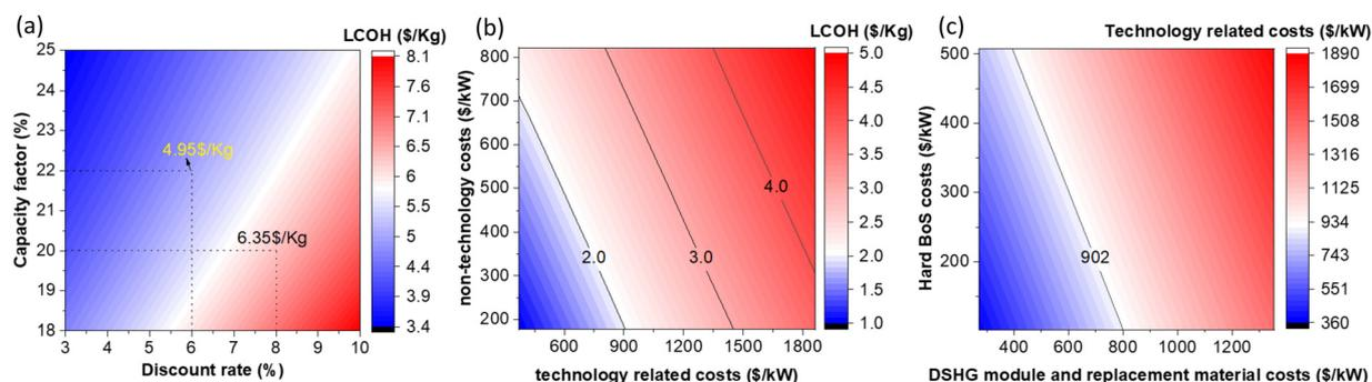
Fig. 5 Contour plot of LCOH of decoupled PV-EC as a function of (a) capacity factor and discount rate (b) non-technology (soft BoS + labour) and technology (hard BoS + DSHG module + replacement materials) related costs. (c) Contour plot of technology related costs as a function of Hard BoS and DSHG module + replacement materials cost.
