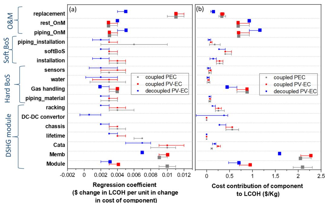
Fig. 3 (a) Estimated regression coefficients for each component considered in DSHG system (b) cost contribution of component to LCOH in \$ per kg assuming baseline LCOH and component cost. Components that have the biggest impact on the LCOH are highlighted with larger markers.
