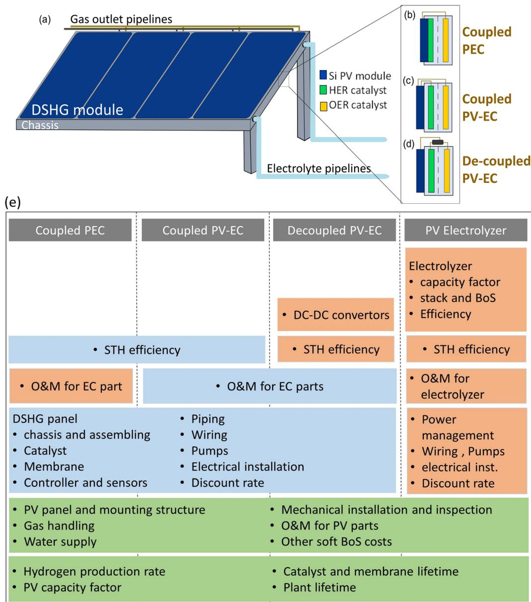
**Fig. 1** Schematic of (a) direct solar hydrogen generation (DSHG) module. Different configurations analysed (b) coupled PEC, (c) coupled PV-EC and, (d) decoupled PV-EC DSHG. (e) Cost breakdowns for all three DSHG system configurations and off grid PV-Electrolyser. Operating conditions and component costs that are identical to all the four systems are shown in green. Costs common in two or more systems are shown in blue and orange shows the costs specific to each system.
