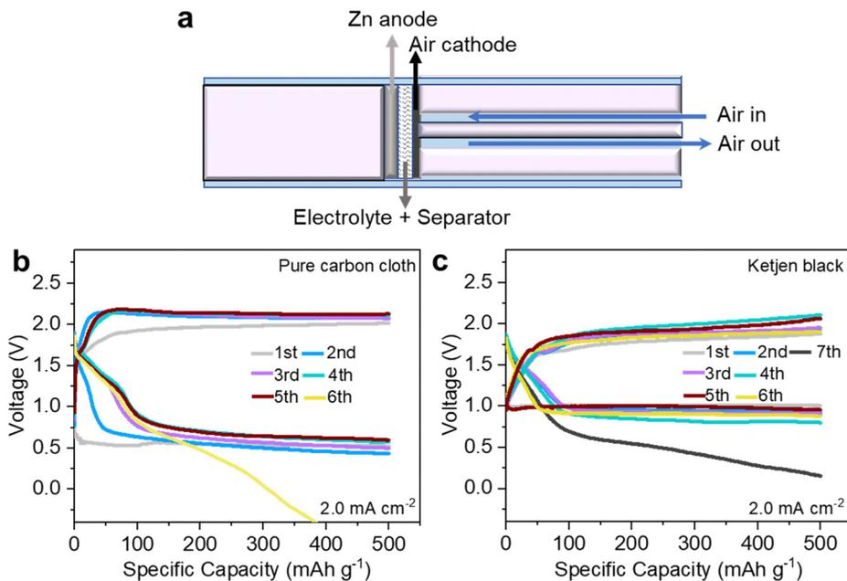
Fig. 1 Schematic illustration and photograph of (a) the bulky Swagelok-type NNZAB; the cycling performance of NNZABs with pure carbon cloth (b) and ketjen black (c) as the cathode.
