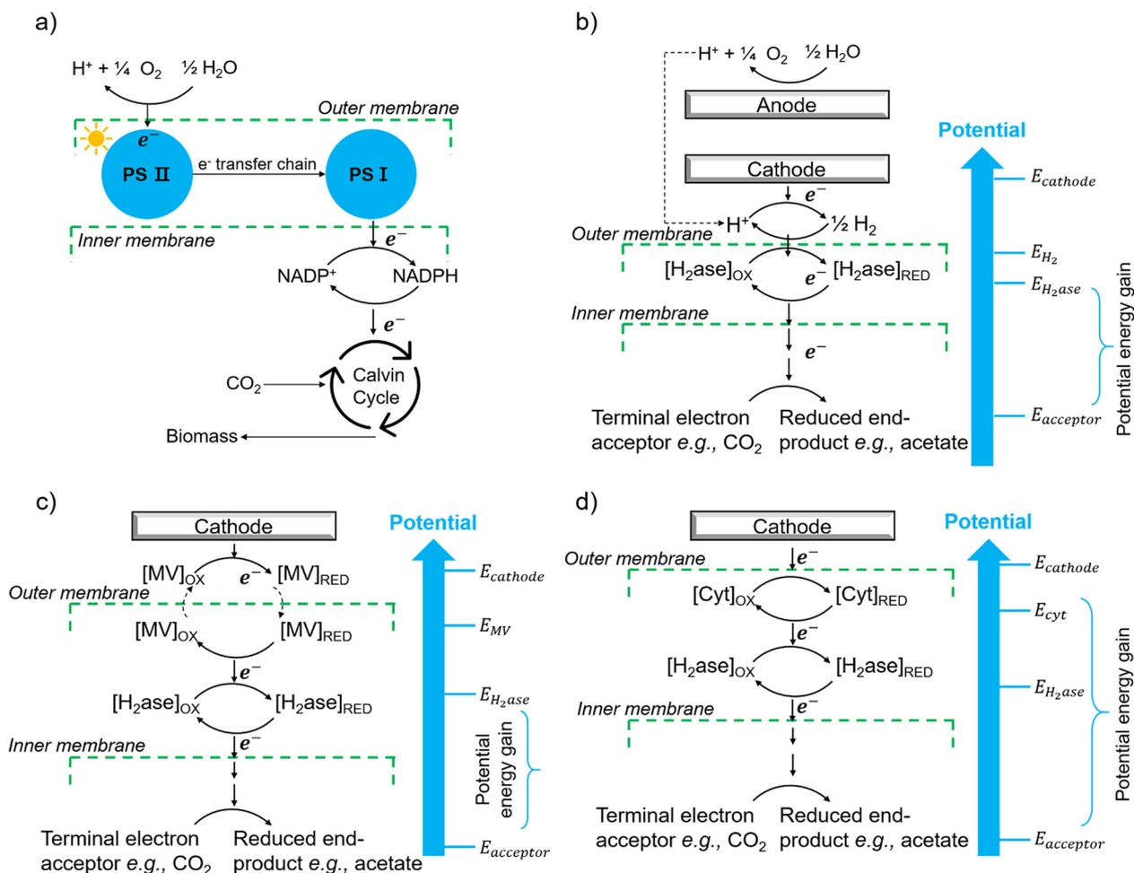
Fig. 6 (a) The process of natural photosynthesis.<sup>122</sup> (b) Proposed cathodic EET mechanism through hydrogen and associated microbial energy gains.<sup>123</sup> (c) Mediated electron transfer through methyl viologen (MV) to a hydrogenase.<sup>126</sup> (d) Direct electron transfer involving cytochrome-hydrogenase partnerships.<sup>137</sup>
