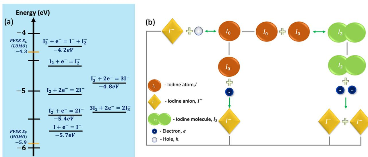
Fig. 2 (a) Approximate positions of iodine/triiodide/diiodide/iodide reduction/oxidation potentials in acetonitrile relative to the valence and conduction bands of the MAPbI<sub>3</sub> perovskite. (b) The reaction cycle considered in the simulation includes iodine atoms (I<sup>0</sup>), iodide anions (I<sup>-</sup>), iodine molecules (I<sub>2</sub>), and electrons and holes. The green arrows mark the reactions' directions.
