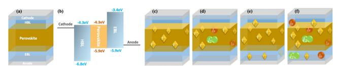
Fig. 1 The simulated scenarios: (a) a solar cell without free iodides, as a reference (c) a solar cell in which the iodides cannot penetrate the blocking layers, (d) a solar cell in which the iodides cannot penetrate the blocking layers but can react, (e) a solar cell in which the iodides penetrate the blocking layers (f) a solar cell in which the iodides penetrate the blocking layers and can react, (b) the materials' energy levels.
