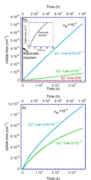
Fig. 5 Simulated time evolution of the iodide density loss for a device biased at 0.9 V and under 1 sun. (a) Conductive blocking layers ( $\mu_{BL} = 10^{-3} \text{ cm}^2 \text{ V}^{-1} \text{ s}^{-1}$ ) (b) resistive blocking layers ( $\mu_{BL} = 10^{-4} \text{ cm}^2 \text{ V}^{-1} \text{ s}^{-1}$ ). The loss is due to the assumption that  $I_2$  is lost through bubbling out.
