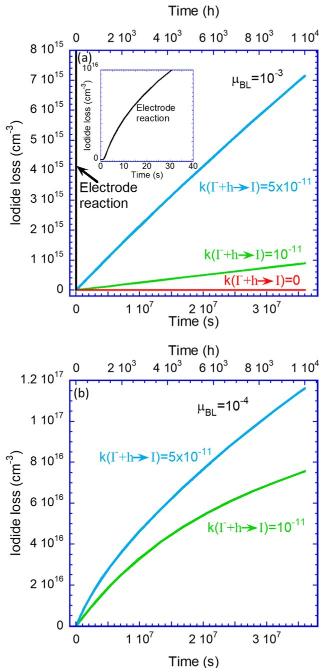
Fig. 5 Simulated time evolution of the iodide density loss for a device biased at 0.9 V and under 1 sun. (a) Conductive blocking layers ( $\mu_{\text{BL}} = 10^{-3} \text{ cm}^2 \text{ V}^{-1} \text{ s}^{-1}$ ) (b) resistive blocking layers ( $\mu_{\text{BL}} = 10^{-4} \text{ cm}^2 \text{ V}^{-1} \text{ s}^{-1}$ ). The loss is due to the assumption that  $\text{I}_2$  is lost through bubbling out.
