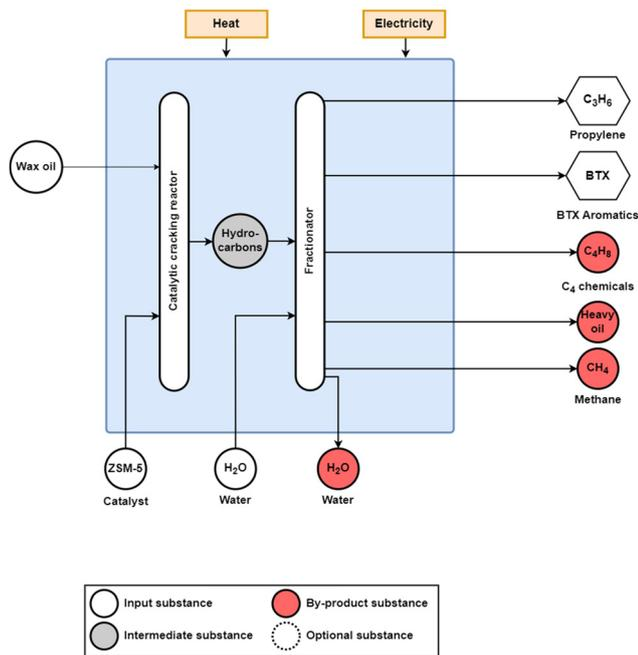
Fig. 5 Deep catalytic cracking of refinery oil for propylene production from wax oil using a zeolite (ZSM-5) catalyst. In addition to the propylene and BTX products, C<sub>4</sub> chemicals, heavy oil, and methane are also produced. Adapted from Zhao *et al.*<sup>24</sup> and Gholami *et al.*<sup>27</sup>
