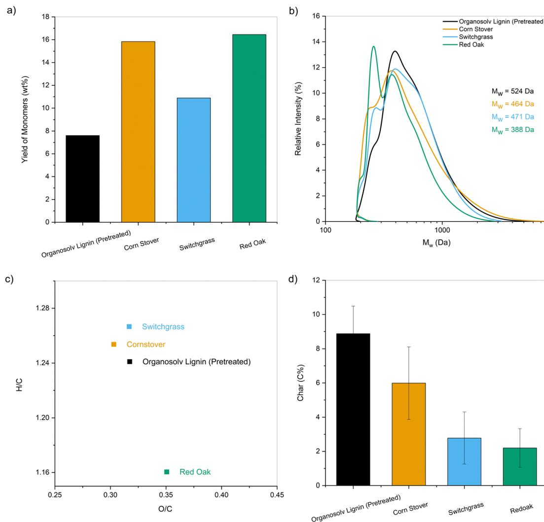
**Fig. 10** Characterization of the pretreated lignin oil obtained from the one-pot fractionation and pretreatment of whole biomass at 250 °C in EtOH over Pd/C. (a) Yield of monomers (wt%) relative to lignin content present in the starting biomass; (b) molecular weight distributions along with their average M<sub>w</sub>; (c) Van Krevelen diagram; (d) char yields (C%) obtained after fast pyrolysis at 500 °C. The results for pretreated organosolv lignin are also provided for comparison.
