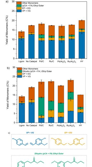
Fig. 6 Yields of phenolic monomers (C%) obtained for the fast pyrolysis at 500 °C of lignin and samples pretreated in EtOH at (a) 200 °C and (b) 250 °C in the presence of various catalysts. (c) Molecular structures of the corresponding monomeric products.
