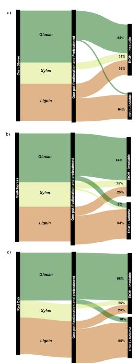
Fig. 9 Component balance (upper bound values) for the products obtained from the one-pot fractionation and pretreatment of whole biomass in EtOH at 250 °C using Pd/C for (a) corn stover, (b) switchgrass, and (c) red oak. The corresponding component balances with the lower bound values are presented in Fig. S8 (ESI†).
