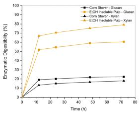
Fig. 13 Enzymatic digestion performed on EtOH-insoluble pulp and untreated corn stover as a control experiment at a digestion time of 72 h.
