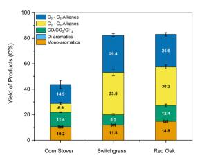
Fig. 12 Carbon yields of products obtained from HDO of the watersoluble fraction recovered after 'one-pot' fractionation and pretreatment of whole biomass. Conditions: MoO<sub>3</sub> catalyst, fast pyrolysis: 500 °C, catalytic upgrading: 400 °C, catalyst:volatile = 40:1.
