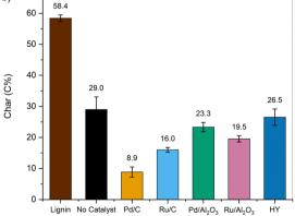
Fig. 5 Char yields (in C%) measured after fast pyrolysis at 500 °C of the parent lignin and lignin samples pretreated in EtOH at (a) 200 °C and (b) 250 °C in the presence of various catalysts.
