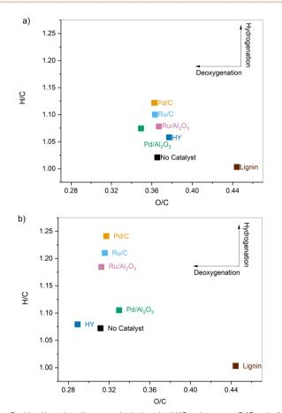
Fig. 2 Van Krevelen diagrams depicting the H/C ratio versus O/C ratio for organosolv lignin and the samples pretreated in EtOH at (a) 200 °C and (b) 250 °C in the presence of various catalysts.
