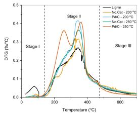
Fig. 4 DTG curves of lignin and representative pretreated samples.
