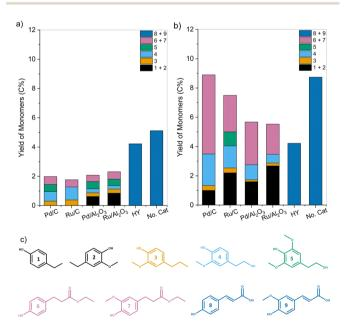
Yield of phenolic monomers (C%) obtained after subjecting organosolv corn stover lignin to a 3 hour pretreatment in EtOH in the presence of various catalysts at (a) 200 °C and (b) 250 °C. (c) The monomeric products consist of (1) ethyl phenol, (2) ethyl guaiacol, (3) 4-propyl guaiacol, (4) propanol guaiacol, (5) 4-(3-hydroxypropyl)-2,6-dimethoxyphenol, (6) ethyl 3-(4-hydroxyphenyl) propanoate, (7) ethyl 3-(4-hydroxy-3-methoxyphenyl) propanoate, (8) p-coumaric acid, (9) ferulic acid.
