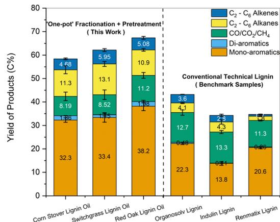
Fig. 11 Carbon yields of products obtained from HDO of the lignin samples after 'one-pot' fractionation and pretreatment of whole biomass. Results obtained with conventional technical lignin samples are also provided for comparison. Conditions: MoO<sub>3</sub> catalyst, fast pyrolysis: 500 °C, catalytic upgrading: 400 °C, catalyst : volatile = 40 : 1.
