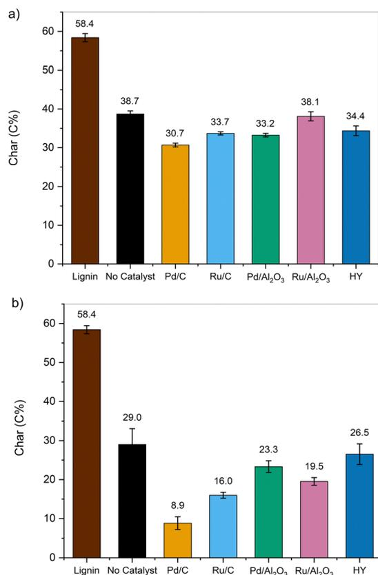
Fig. 5 Char yields (in C%) measured after fast pyrolysis at 500 °C of the parent lignin and lignin samples pretreated in EtOH at (a) 200 °C and (b) 250 °C in the presence of various catalysts.
