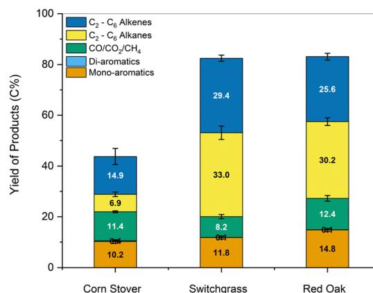
Fig. 12 Carbon yields of products obtained from HDO of the water-soluble fraction recovered after 'one-pot' fractionation and pretreatment of whole biomass. Conditions: MoO<sub>3</sub> catalyst, fast pyrolysis: 500 °C, catalytic upgrading: 400 °C, catalyst : volatile = 40 : 1.
