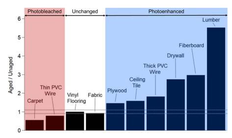
Fig. 3 Ratios of the 2 h aged to unaged integrated, visible range MAC values. The reported ratios were calculated by integrating the MAC values in the visible range (400–700 nm) then referencing the 2 h aged, integrated MAC value to that of the unaged, integrated MAC value. The shading color corresponds to classification of OA into three categories: photobleached (red), unchanged (white) and photoenhanced (blue). The dashed line (0.9 to 1.1) indicates the threshold for the unchanged category.
