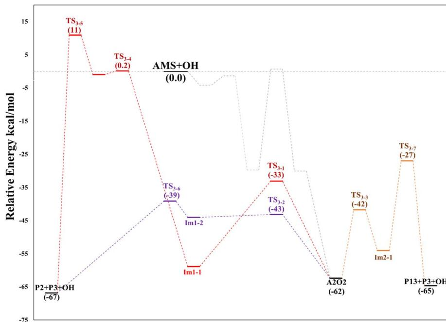
Fig. 12 Relative energy diagram for decomposition of the A2O2 intermediate (addition to C2) formed in the AMS oxidation initiated by OH radicals in the absence of NO<sub>x</sub> at the M06-2X/GD3/aug-cc-pVTZ level.
