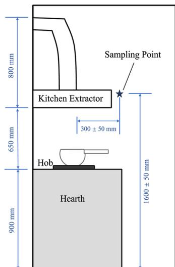
Fig. 1 Schematic layout and location of sampling point in the studied kitchens.
