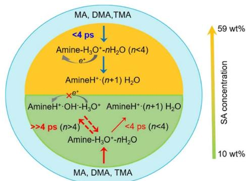
Fig. 6 Methylamines participate in two types of reactions at low and high SA concentrations.<sup>2</sup>
