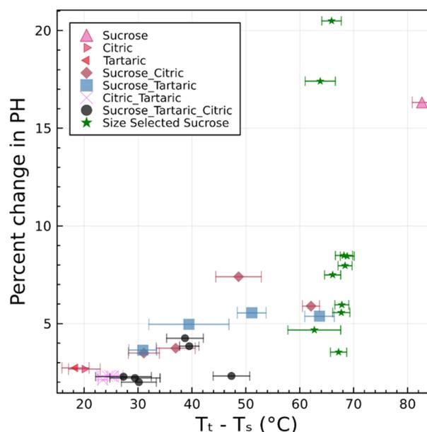
Fig. 8 Summary of the observed change in digitizer PH during the phase transition for all measurements.  $T_s$  is the system temperature which for these experiments are  $\sim 8$  °C. The line and shading show the linear regression and associated uncertainty of the slope.
