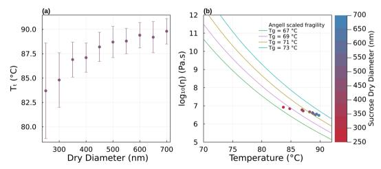
Fig. 5 (a) Transition temperature for pure sucrose particles as a function of dry diameter. Error bars show the standard deviation of the logistic fit (eqn (2)). (b) Derived viscosity at the transition temperature based on particle diameter as described in Section 2.2 vs. the measured transition temperature. Symbol colors denote the particle dry diameter. Model lines correspond to D = 4.8. Line color corresponds to different  $T_{\rm q}$  values.
