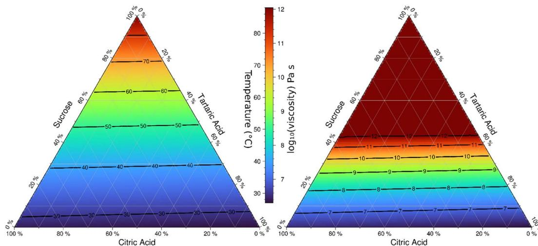
Fig. 9 (Left) False color representation and contours of the predicted transition temperature for  $\eta = 6.9 \times 10^6$  Pa s for ternary compositions of citric acid, sucrose, and tartaric acid. Color and values on contours correspond to temperature in °C. (Right) False color representation of viscosity at 30 °C. Colors and values on contours represent  $\log_{10}$  transformed viscosity in Pa s, *i.e.*,  $10 = 10^{10}$  Pa s. Values >12 correspond to glassy phase states.
