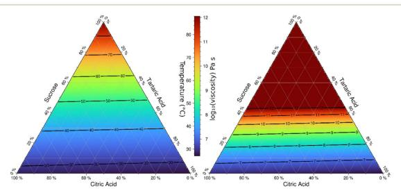
Fig. 9 (Left) False color representation and contours of the predicted transition temperature for  $\eta = 6.9 \times 10^6$  Pa s for ternary compositions of citric acid, sucrose, and tartaric acid. Color and values on contours correspond to temperature in °C. (Right) False color representation of viscosity at 30 °C. Colors and values on contours represent log10 transformed viscosity in Pa s, *i.e.*,  $10 = 10^{10}$  Pa s. Values >12 correspond to glassy phase states.
