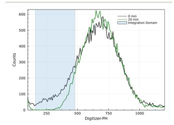
Fig. 2 Example digitizer-PH frequency distributions before (black) and after (green) restructuring. The shaded area illustrates the integration domain in eqn (1). The evaluated  $\mu_{PH}$  between 160 and 480 digitizer-PH is 375 and 440 before and after restructuring, respectively.
