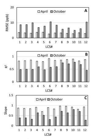
Fig. 5 (A) RMSE, (B)  $R^2$ , and (C) slope values for all 12 sensors over the April 2021 and October 2021 collocation periods at West Phoenix using Model 1.0.
