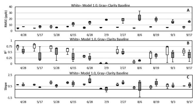
Fig. 4 Box and whisker plots for the (A) RMSE, (B)  $R^2$ , and (C) slope values of the Model 1.0 and Clarity baseline calibrated data from each 2 weeks collocation. Each point is a compilation of values from the 3 collocated sensors for that period. The lines within the boxes represent the medians, the interquartile range is the range of the boxes with the top representing the 75th and the bottom the 25th percentile. The whiskers represent the maximum and minimum values in the data.
