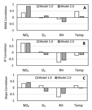
Fig. 7 (A) RMSE, (B)  $R^2$ , and (C) slope correlations for the Model 1.0 and Model 2.0 calibrations to FRM NO<sub>2</sub>, FEM O<sub>3</sub>, internal sensor relative humidity, and internal sensor temperature.
