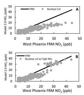
Fig. 1 Comparison of a (A) Buckeye trained calibration and (B) a Buckeye trained calibration including high NO<sub>2</sub> data points applied to Sensor 6 at West Phoenix
