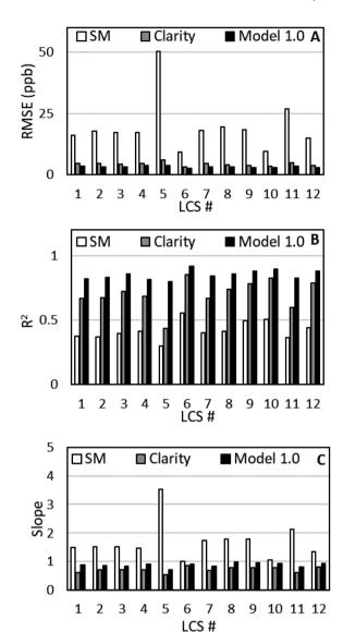
Fig. 2 (A) RMSE, (B)  $R^2$ , and (C) slope values for all 12 sensors based on hourly data over the April 2021 collocation period at West Phoenix using the SM calibration, Clarity Baseline Model, and Model 1.0.
