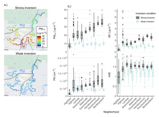
Fig. 5 (a) PM<sub>2.5</sub> map for strong and weak inversion conditions using 50 m grid cell aggregations. Concentration values outside of the colorscale range are given the end values of the range, for visualization purposes. (b) Neighborhood boxplots of PM<sub>2.5</sub>, BC, PN, and AAE for both inversion conditions. Neighborhoods for all pollutants are arranged on the x-axis in order of increasing median PM<sub>2.5</sub> concentration within the strong inversion category.
