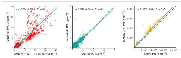
Fig. 9 Comparison of PM, BC, and PN measurements between mobile-suite instruments and stationary instruments at the ALPACA house field site during co-location.
