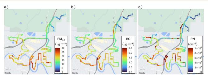
Fig. 2 Mean  $50 \times 50$  m grid cell concentrations across all 29 drives for each of (a) PM<sub>2.5</sub>, (b) BC, and (c) PN. All grid cells shown meet a minimum visit threshold of 10 visits.
