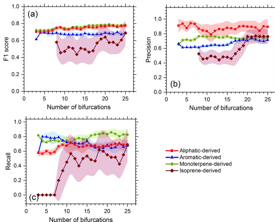
Fig. 2 The overall accuracy of the decision tree model in the precursor apportionment of atmospheric oxygenated organic molecules using laboratory testing data (a) is for *F1-score*, (b) is for *precision*, and (c) is for *recall*. The dotted lines are the mean value of repeated tests and the shaded area illustrates the standard deviation.
