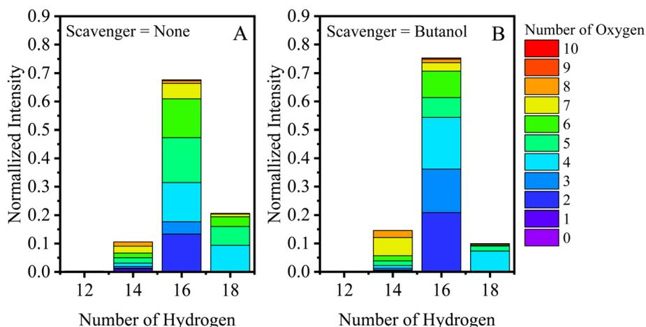
Fig. 2 Hydrogen distribution plotted for C<sub>10</sub>H<sub>x</sub>O<sub>y</sub> molecules (30 min after  $\alpha$ -pinene addition), and colored according to the number of oxygen atoms present for an experiment (A) without an OH scavenger, and (B) with butanol present as a scavenger.
