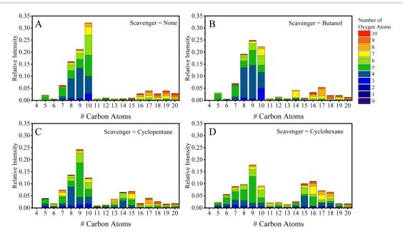
Fig. 1 (A-D) Data from EESI-TOF binned according to number of carbon atoms (x-axis) and number of oxygen atoms at the time of maximum SOA mass concentration during an  $\alpha$ -pinene ozonolysis experiment with (A) no scavenger present, (B) butanol present, (C) cyclopentane present, and (D) cyclohexane present.
