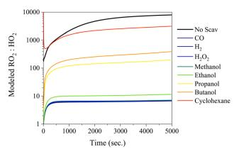
Fig. 4 RO<sub>2</sub>: HO<sub>2</sub> ratio modelled using a box model based on MCM v3.3.1 for:  $\alpha$ -pinene 25 ppb,  $O_3$  250 ppb, and excess concentration of the scavenger (CO -  $30\,000$  ppm,  $H_2$  - 2%,  $H_2O_2$  - 200 ppm, methanol – 200 ppm, ethanol – 200 ppm, n-propanol – 200 ppm, nbutanol - 200 ppm, and cyclohexane - 200 ppm).
