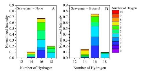
Fig. 2 Hydrogen distribution plotted for  $C_{10}H_xO_y$  molecules (30 min after  $\alpha$ -pinene addition), and colored according to the number of oxygen atoms present for an experiment (A) without an OH scavenger, and (B) with butanol present as a scavenger.
