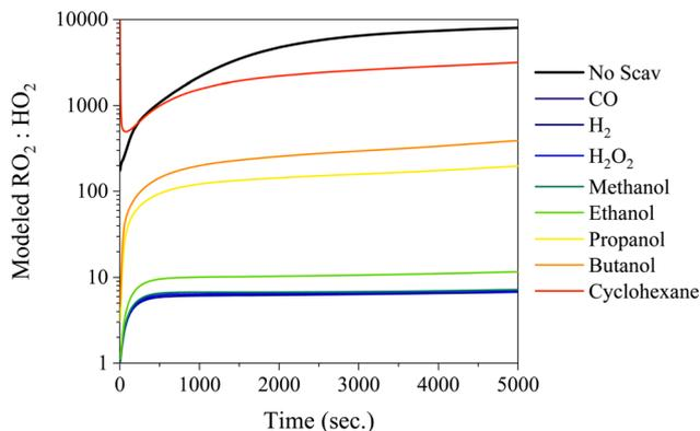
Fig. 4  $\text{RO}_2 : \text{HO}_2$  ratio modelled using a box model based on MCM v3.3.1 for:  $\alpha$ -pinene 25 ppb,  $\text{O}_3$  250 ppb, and excess concentration of the scavenger (CO – 30 000 ppm,  $\text{H}_2$  – 2%,  $\text{H}_2\text{O}_2$  – 200 ppm, methanol – 200 ppm, ethanol – 200 ppm, *n*-propanol – 200 ppm, *n*-butanol – 200 ppm, and cyclohexane – 200 ppm).
