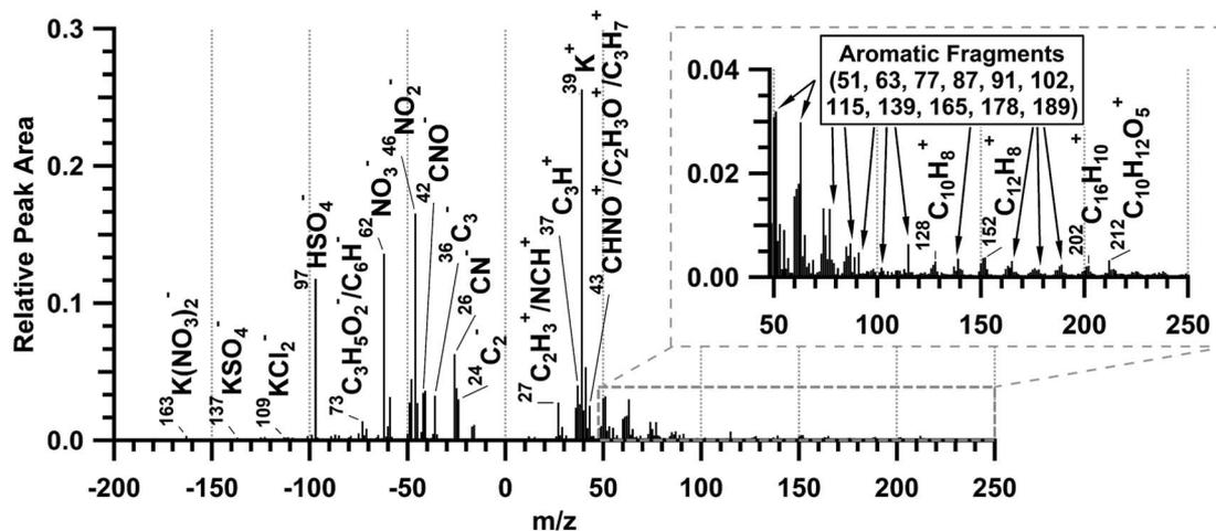
Fig. 5 ATOFMS average positive and negative ion mass spectrum of 5500 freshly emitted biomass burning particles sampled during plumes 1–6.
