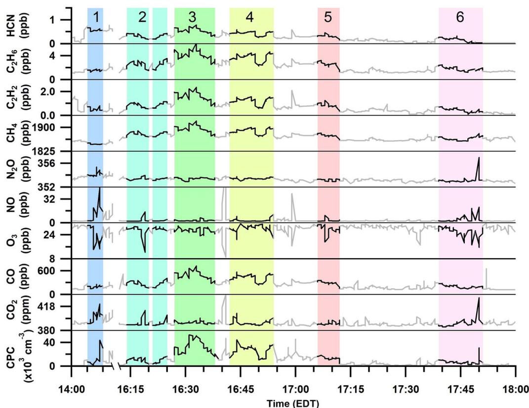
Fig. 2 Time series of 20 s averaged  $\text{HCN}$ ,  $\text{C}_2\text{H}_6$ ,  $\text{C}_2\text{H}_2$ ,  $\text{CH}_4$ ,  $\text{N}_2\text{O}$ ,  $\text{NO}$ ,  $\text{O}_3$ ,  $\text{CO}$ , and  $\text{CO}_2$  mole ratios and total particle (CPC) number concentrations over the full prescribed burn sampling period. Identified periods of smoke plume sampling are highlighted and numbered. Areas that are greyed out were not included in the plume analyses (Table 2).
