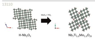
Structural and electrochemical insights into novel Wadsley Roth  $Nb_7Ti_{1.5}Mo_{1.5}O_{25}$  and  $Ta_7Ti_{1.5}Mo_{1.5}O_{25}$  anodes for Li-ion battery application
