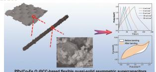
A crosslinked network polypyrrole coated cobalt doped  $Fe_2O_3$ @carbon cloth flexible anode material for quasi-solid asymmetric supercapacitors
