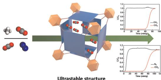
Efficient separation of CO<sub>2</sub> from CH<sub>4</sub> and N<sub>2</sub> in an ultra-stable microporous metal–organic framework
