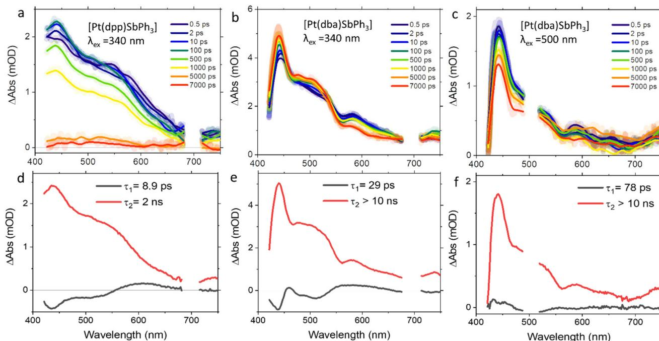
**Fig. 7** Transient absorption spectra (TAS) at selected delay times (a–c) and decay-associated spectra (d–f) for [Pt(dpp)(SbPh<sub>3</sub>)] following excitation at 340 nm (a and d), [Pt(dba)(SbPh<sub>3</sub>)] upon excitation at 340 nm (b and e) and 500 nm (c and f) in THF. The thicker lines in TAS shows smoothed data.
