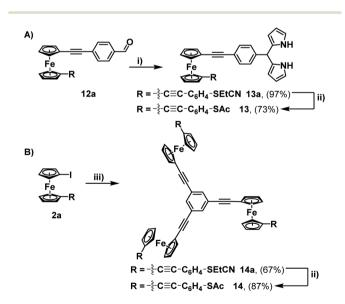
Scheme 5 (A) Synthesis of 13 and (B) synthesis of 14. Reaction conditions: (i) pyrrole, TFA, RT, 4 hours; (ii) NaOMe (25% in MeOH), THF, 30 min followed by  $Ac_2O$  30 min; (iii) 1,3,5-triethynylbenzene, Cul, [Pd  $(CH_3CN)_2Cl_2$ ][PH( $^tBu_3$ ) $_2$ ]BF $_4$ , DIPA, THF, RT, >16 h.
