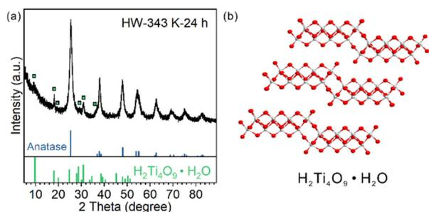
**Fig. 5** (a) XRD patterns of the samples obtained after heating  $\text{TiO}_2(\text{B})$  nanosheets in water dispersion at 343 K for 24 hours; peaks belonging to  $\text{H}_4\text{Ti}_4\text{O}_{10}$  are marked with squares. (b) Crystal structure of  $\text{H}_4\text{Ti}_4\text{O}_{10}$ .
