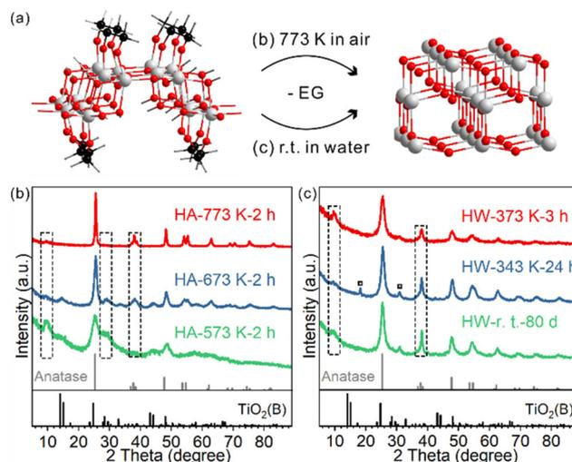
**Fig. 2** (a) Scheme showing the phase transformation from EG-protected  $\text{TiO}_2(\text{B})$  nanosheets to anatase either through heating in air or in water. Colour code: O (red), Ti (grey), C (black), and H (white). XRD patterns of the samples heated at different temperatures (b) in air and (c) in water.
