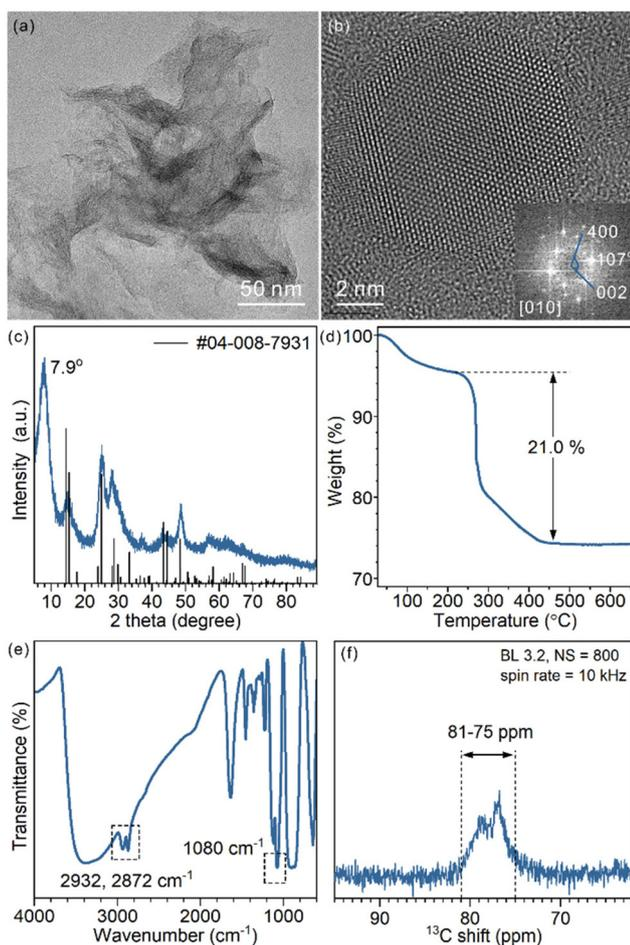
**Fig. 1** (a) Representative TEM image, (b) HRTEM image and FFT pattern, (c) XRD pattern, (d) TGA curve (e) FT-IR spectrum and (f)  $^{13}\text{C}$  ss-NMR spectrum of the as-prepared  $\text{TiO}_2(\text{B})$  nanosheets.
