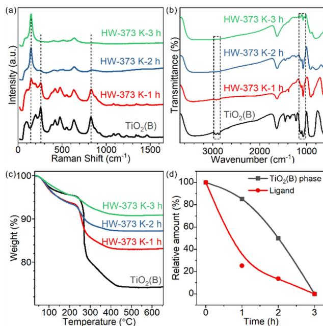
Fig. 3 (a) Raman and (b) FT-IR spectra and (c) TGA results of the  $\text{TiO}_2(\text{B})$  nanosheets and samples obtained after heating in water at 373 K for 1, 2 and 3 hours; and (d) calculated mass ratio of the  $\text{TiO}_2(\text{B})$  phase and residual EG ligand.
