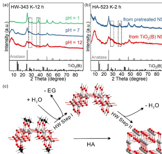
**Fig. 4** XRD patterns of the samples obtained (a) after heating  $\text{TiO}_2(\text{B})$  nanosheets in water dispersion of different pH values at 343 K for 12 hours and (b) after heating the pre-treated and as-prepared  $\text{TiO}_2(\text{B})$  nanosheets in air at 523 K for 2 hours. (c) Scheme showing the surface speciation in the phase transition.
