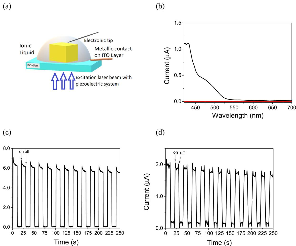
**Fig. 3** (a) Experimental scheme of the single crystal contact; (b) photocurrent spectra of a single crystal of **MoBr** embedded into **BMIMBF<sub>4</sub>** (black line) and a drop of **BMIMBF<sub>4</sub>** as a blank (red line), under excitation with a supercontinuum laser at different wavelengths; (c) **MoBr** and (d) **MoCl** current–time ( $I-t$ ) curves under 405 nm LED light with 0.1 Hz light on/off cycles.
