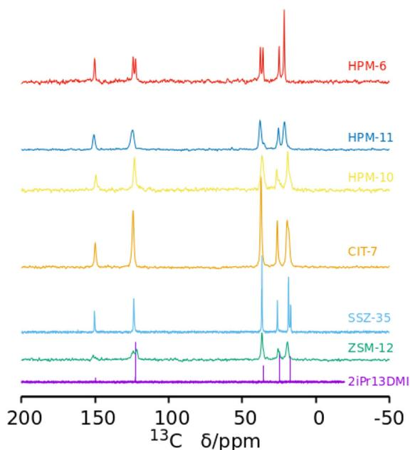
**Fig. 3**  $^{13}\text{C}$  NMR spectrum of 2iPr13DMI iodide in  $\text{D}_2\text{O}$  solution and  $^{13}\text{C}$  MAS NMR spectra of six as-made phases prepared in this work as Ge, increases (from bottom). In the bottom spectrum, the C at position 2 of the aromatic ring (between both N) is barely visible at around 150 ppm. That carbon typically displays a very small relative intensity in the proton-decoupled  $^{13}\text{C}$  NMR spectra of this kind of compound.<sup>56,57</sup>
