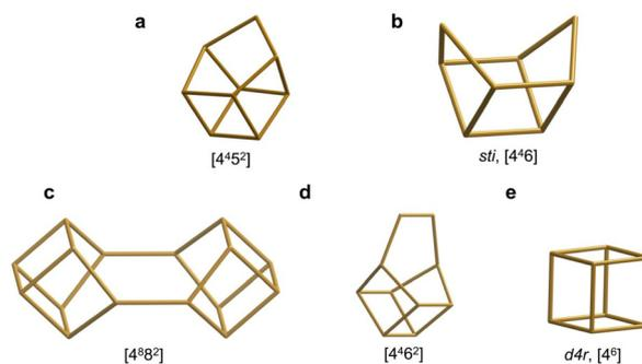
Fig. 5 Several cages that can be formally considered as being derived from the  $d4r$  cage by modification at one corner and which may provide similar environments for fluoride at the opposite side. They appear in CSV (a), STI (b), PKU-22 (c), PKU-26 (d) and, among others, AST (e).<sup>68</sup>
