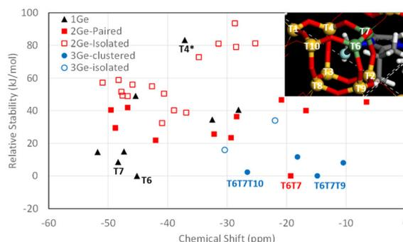
**Fig. 7** Relative stability vs.  $^{19}\text{F}$  NMR chemical shift for  $\text{F}^-$  in  $[4^45^2]$  cages with 1 Ge (black triangles), 2 Ge (red squares) in paired (solid) or isolated (empty) positions and 3 Ge (blue circles) in clustered (solid) or non-clustered (empty) positions. Relative stabilities are calculated independently for 1Ge, 2Ge and 3Ge systems. The inset shows the labels for the T atoms in the  $[4^45^2]$  cage, with 2Ge in T6 and T7 positions.
