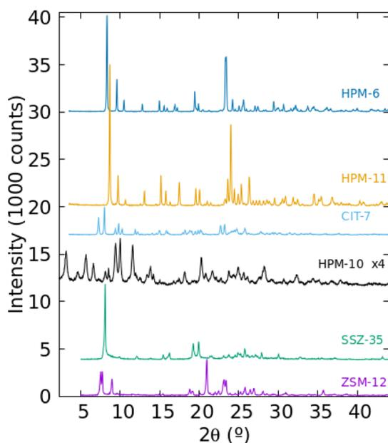
**Fig. 2** Powder XRD of the six zeolitic phases synthesized as pure phases in this work as Ge<sub>f</sub> in the gel increases (from bottom to top).
