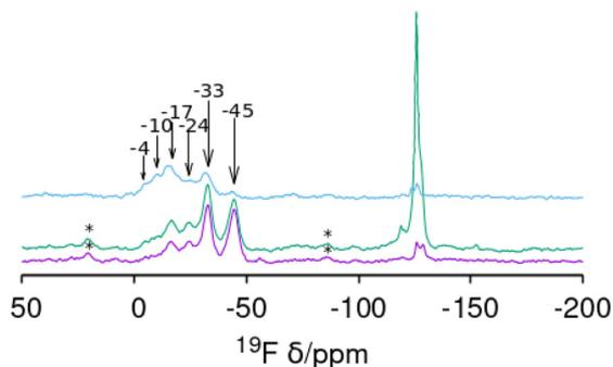
**Fig. 8**  $^{19}\text{F}$  MAS NMR spectra of CSV samples synthesized at  $\text{Ge}_f$  equal to (from bottom) 0.09, 0.1 and 0.2. The resonances around  $-115$  to  $-130$  ppm are assigned to impurities. Spinning side bands are marked with \*. Measured chemical shifts are signaled by arrows.
