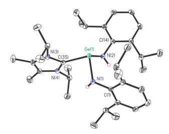
Fig. 1 Molecular structure of NHC  $\rightarrow$  Ge[N(H)Ar]<sub>2</sub> (1). Ellipsoids are drawn at 30% probability. H atoms except for NH groups have been omitted for clarity. Selected bond lengths (Å) and bond angles (°): Ge(1)–C(35) 2.144(2), Ge(1)–N(1) 1.951(2), Ge(1)–N(2) 1.950(2); N(1)–Ge(1)–N(2) 97.04(9), N(1)–Ge(1)–C(35) 89.75(8), N(2)–Ge(1)–C(35) 101.40(8).
