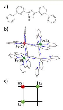
Fig. 1 (a) Pyrazole-bridged compartmental ligand HL. (b) Molecular representation of the  $[Fe_3L_4]^{4+}$  grid. Fe(A)and Fe(B) ions are in the LS state, and Fe(C) ions are in the HS state. Counter ions, solvent molecules and hydrogen atoms are omitted for clarity. (c) Schematic representation of the grid in FE3.
