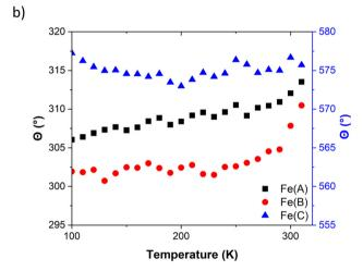
Fig. 2 Temperature dependence of (a) (Fe-N) bond length distances and (b) angular distortions ( $\Theta$ ) in FE3. Values for Fe(A) and Fe(B) share the same axis
