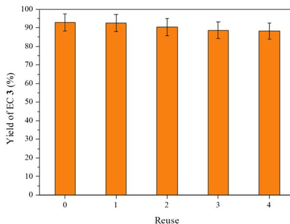
Fig. 5 Reuses of MOF **1** (6 mol%) as a catalyst for the cycloaddition reaction of ethylene oxide (EO, **2**) dissolved in THF (1.6 M) to give ethylene carbonate (EC, **3**) with TOAB (2 mol%) under 25 bar of CO<sub>2</sub> at 120 °C for 4 h. Error bars account for 5% uncertainty.
