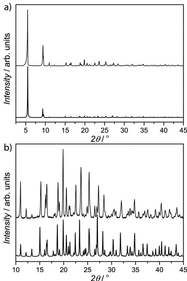
**Fig. 3** (a) Calculated (bold lines) and experimental (solid lines) PXRD pattern profiles of **1** in the  $2\theta$  range of 2.0–45.0° at room temperature, and an enlarged image in the range of 10.0–45.0° (b).
