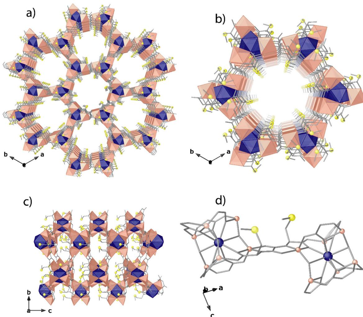
**Fig. 1** Perspective views of the porous networks of **1** (a) and a single channel along the *c* (a and b) and *a* (c) axes. Perspective view of the  $\{Zn_2[(S,S)\text{-Mecysmox}]\}$  dimer connecting  $Sr^{II}$  cations (d). Colour code: Zn, Sr and S atoms are represented by salmon polyhedra, blue polyhedra, and yellow spheres, respectively, whereas the ligands (except sulphur) are depicted as gray sticks.
