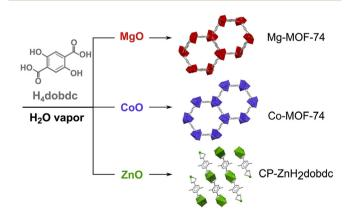
Scheme 2 Products obtained by the reaction of different metal oxides with  $H_4$ dobdc in a humid atmosphere at 130 °C. For MgO and CoO, MOF-74 is obtained (CCDC: VOGTIV and ORIWAP, respectively). ZnO yields a dense coordination polymer  $[Zn(H_2O)_2(H_2dobdc)]_n$  (CCDC: ODIPOH01).
